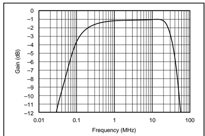
FIGURE 13. Simulated Frequency Response for Differential Filter.
