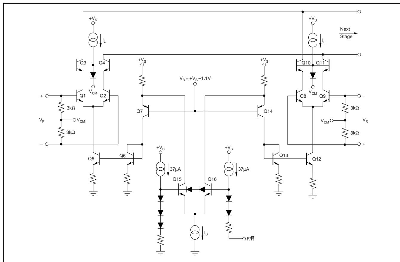
FIGURE 7. Input Stage Schematic (1 of 4 channels).
