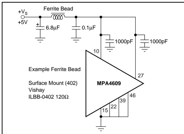
FIGURE 15. Power Supply PI Filter for Improved PSRR.
