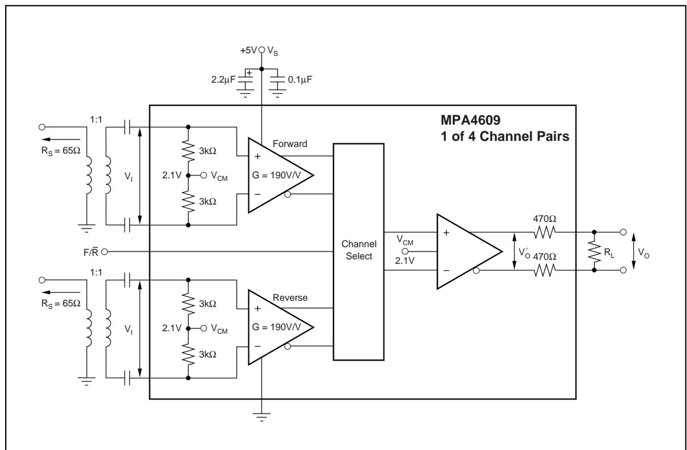
FIGURE 1. Typical Test Circuit for 1 of 4 Channel Pairs.
