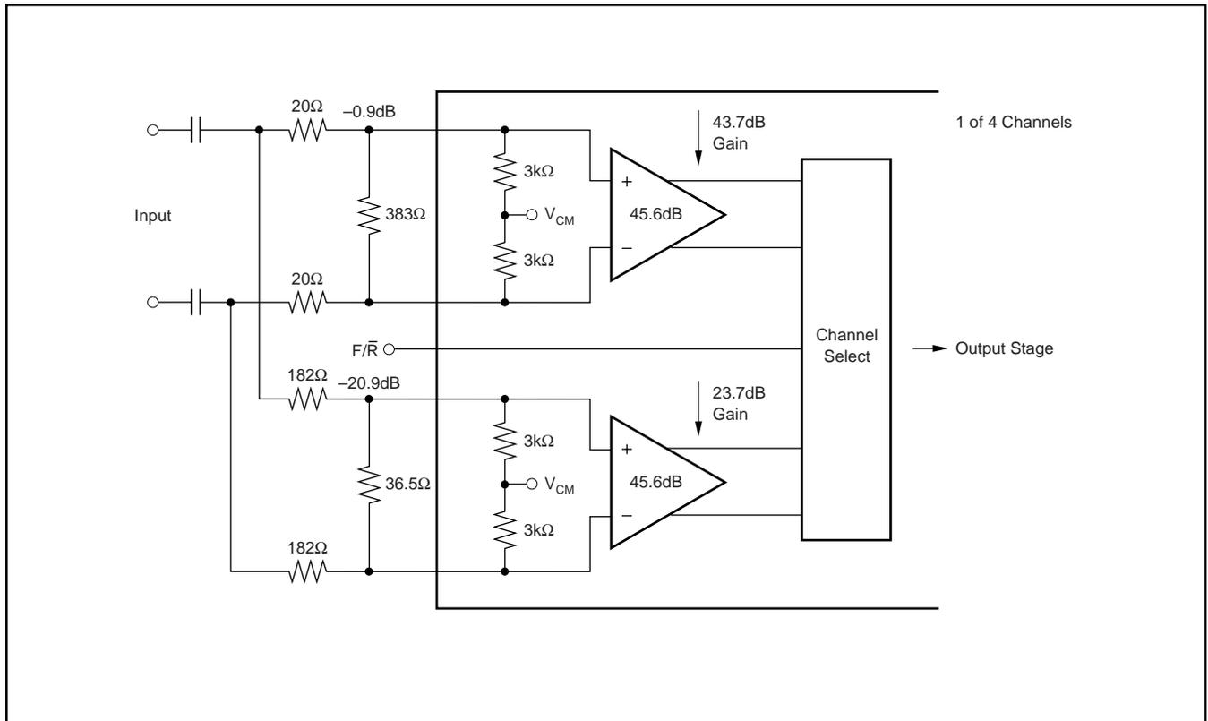
FIGURE 4. Switched Attenuator to Increase ADC Dynamic Range.
