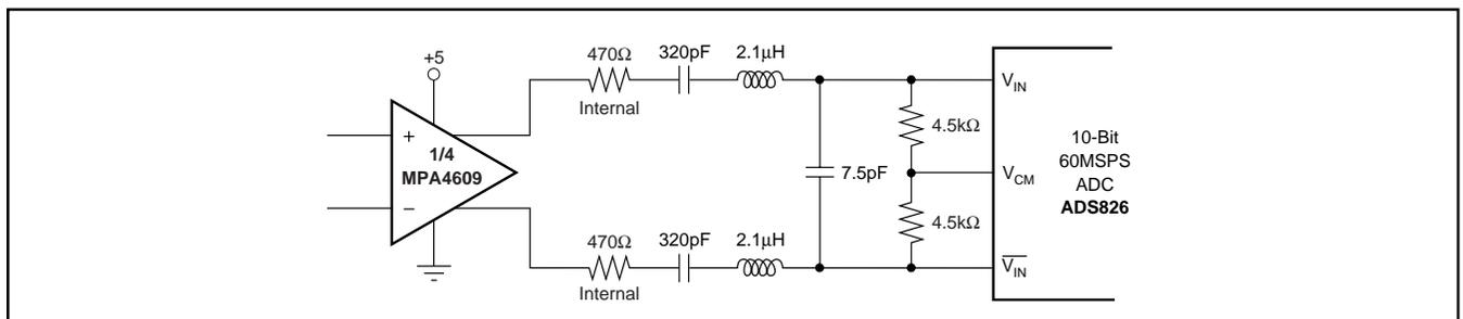
FIGURE 12. 3rd-Order Filter to Improve Harmonic Distortion.
