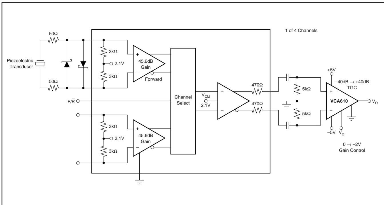
FIGURE 6. Sonar Amplifier with Time Gain Control.
