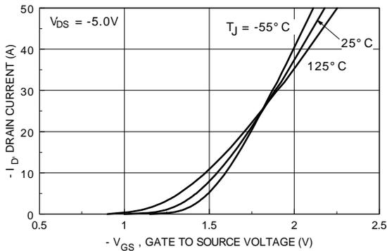
Figure 5. Transfer Characteristics.
