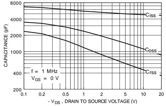
Figure 8. Capacitance Characteristics.
