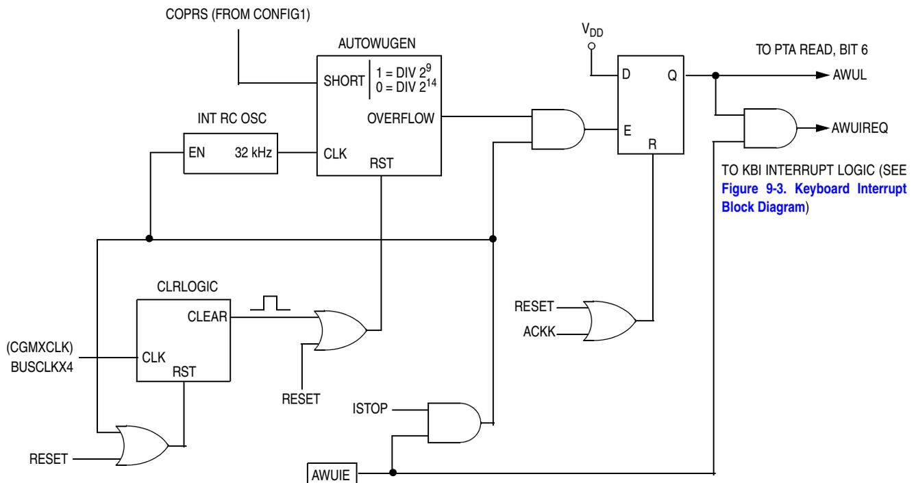
**Figure 4-2. Auto Wakeup Interrupt Request Generation Logic**
