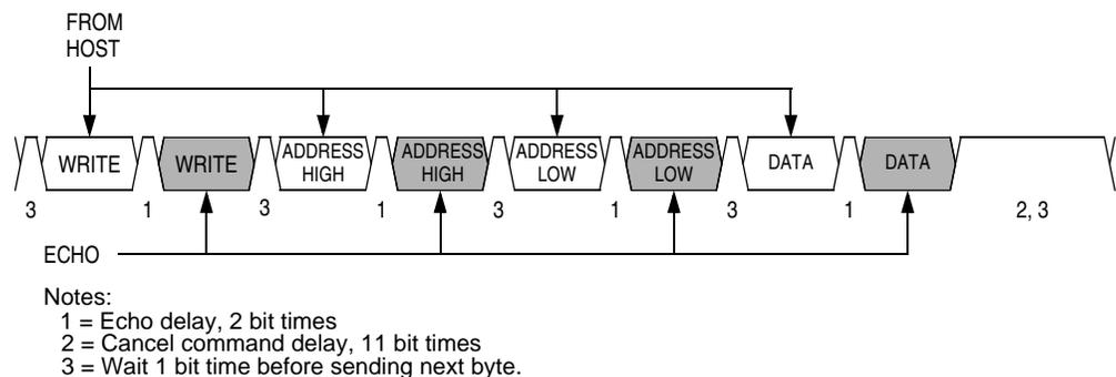
Figure 15-17. Write Transaction
