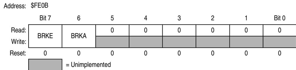
**Figure 15-4. Break Status and Control Register (BRKSCR)**
