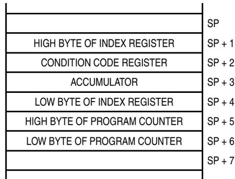
**Figure 15-18. Stack Pointer at Monitor Mode Entry**
