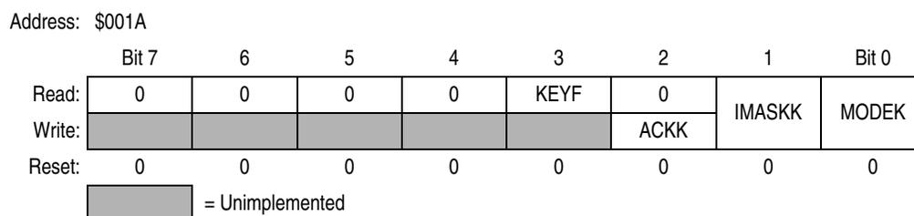
**Figure 4-4. Keyboard Status and Control Register (KBSCR)**
