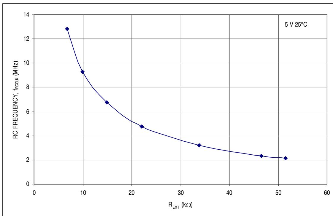
Figure 16-4. RC versus Frequency (5 Volts @ 25°C)
