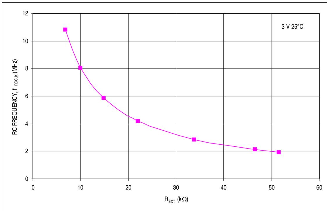
Figure 16-8. RC versus Frequency (3 Volts @ 25°C)
