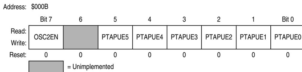
**Figure 12-5. Port A Input Pullup Enable Register (PTAPUE)**
