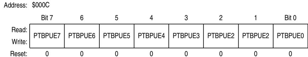
**Figure 12-9. Port B Input Pullup Enable Register (PTBPUE)**
