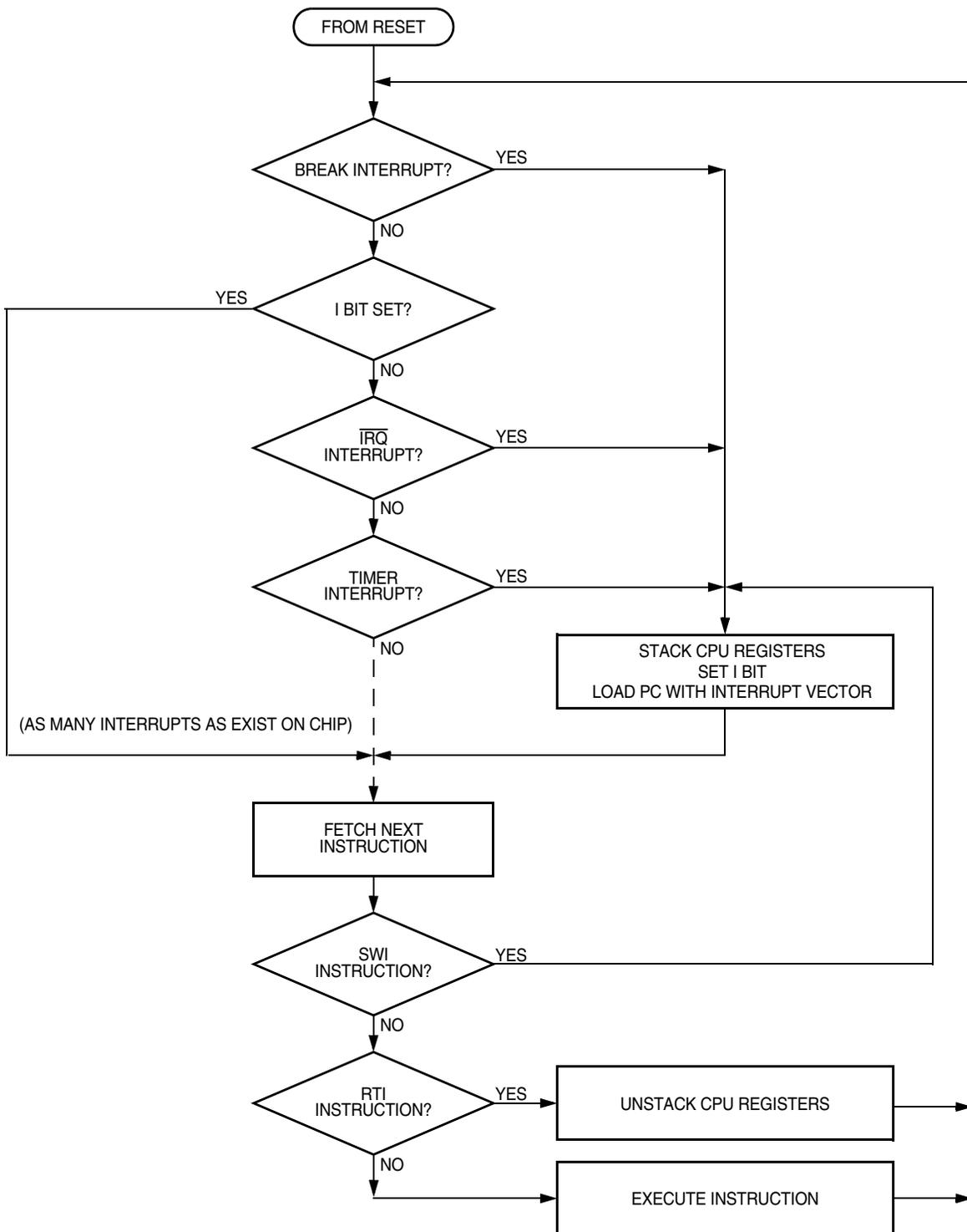
Figure 13-8. Interrupt Processing
