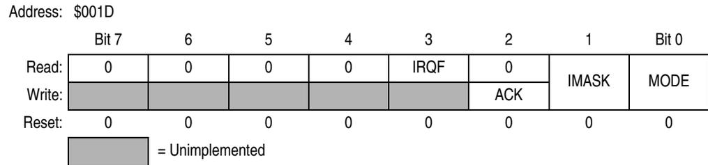
**Figure 8-4. IRQ Status and Control Register (INTSCR)**
