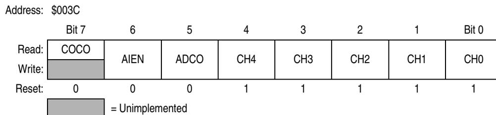
**Figure 3-4. ADC Status and Control Register (ADSCR)**
