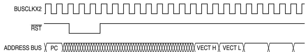
**Figure 13-4. External Reset Timing**
