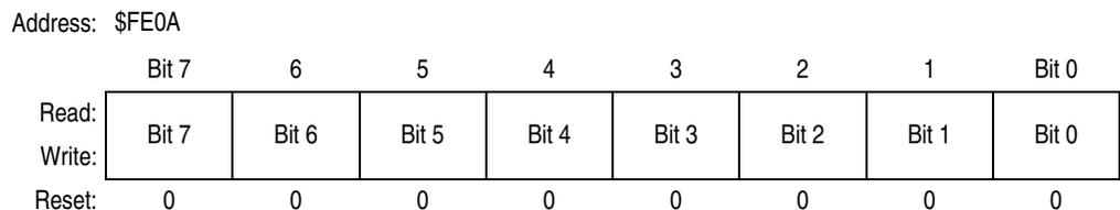
**Figure 15-6. Break Address Register Low (BRKL)**
