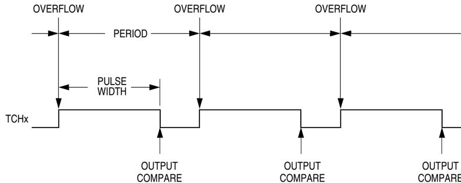
**Figure 14-4. PWM Period and Pulse Width**
