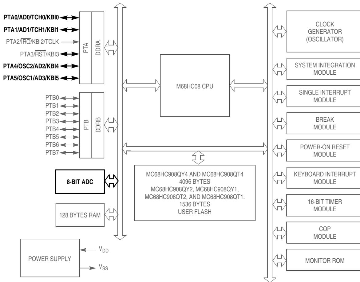
$\overline{RST}$ ,  $\overline{IRQ}$ : Pins have internal (about 30K Ohms) pull up
