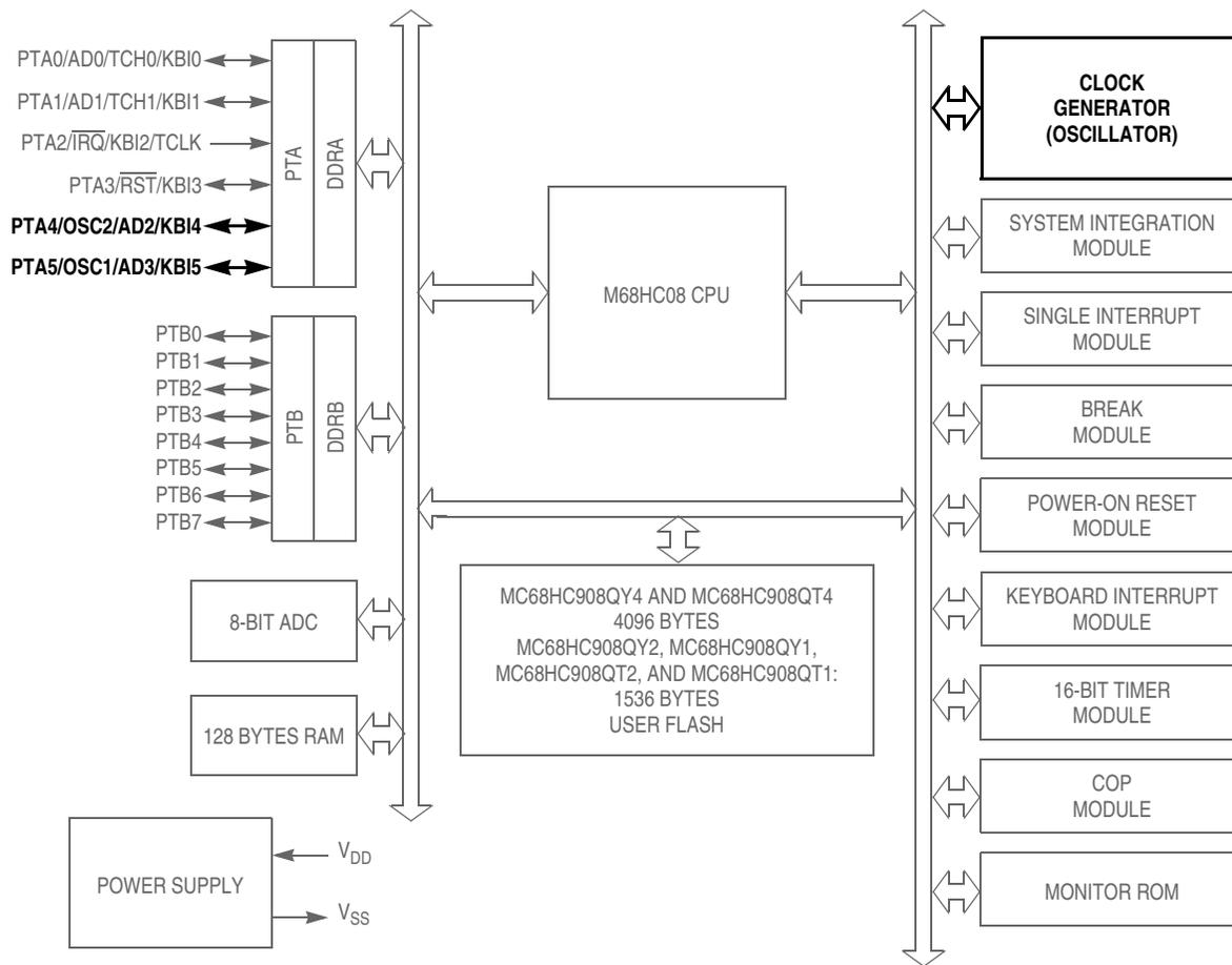
$\overline{\text{RST}}$ ,  $\overline{\text{IRQ}}$ : Pins have internal (about 30K Ohms) pull up
