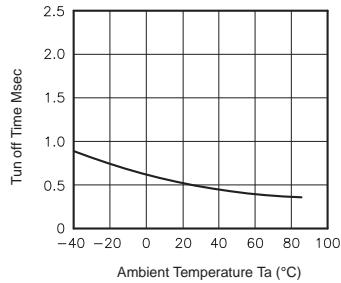
**Fig.5** LED operate vs. ambient temperature
