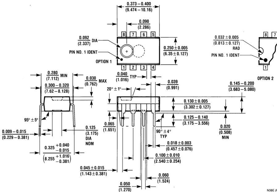
**8-Lead (0.300" Wide) Molded Dual-In-Line Package**
