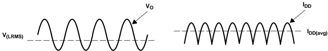
Figure 41. Voltage and Current Waveforms for BTL Amplifiers
