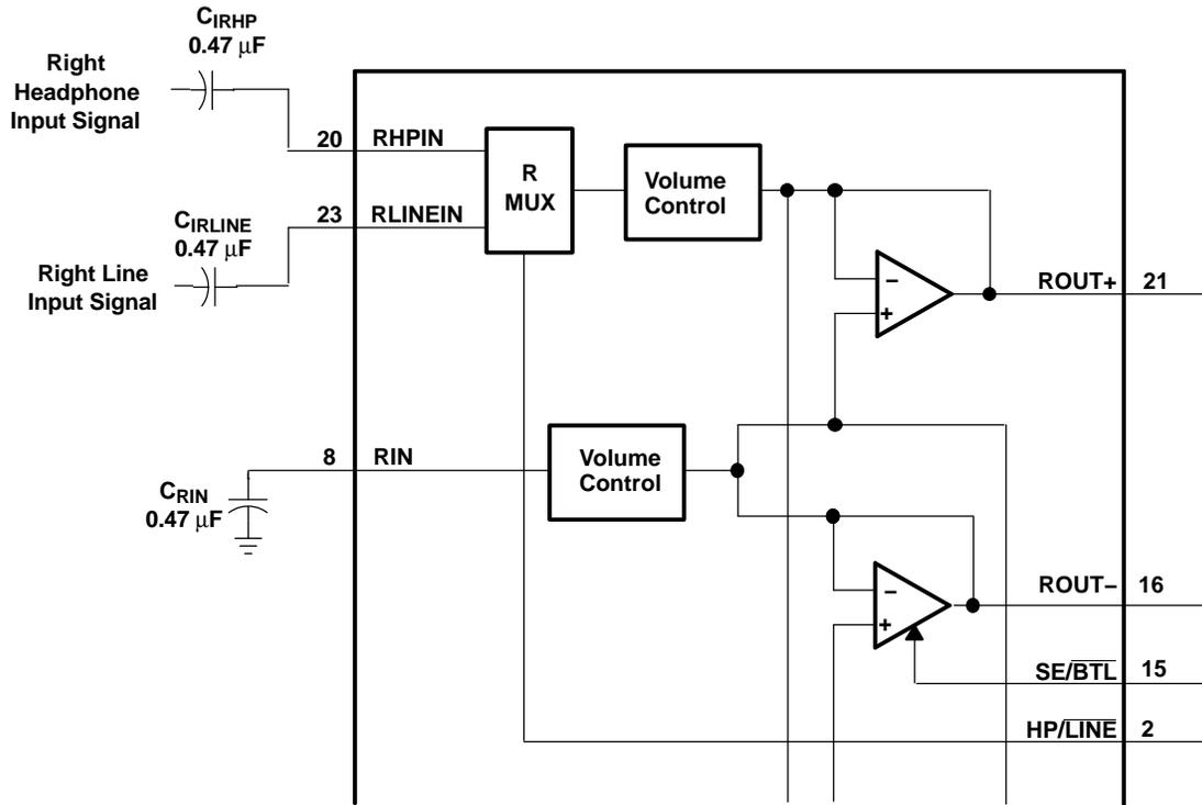
**Figure 43. TPA0312 Example Input MUX Circuit**
