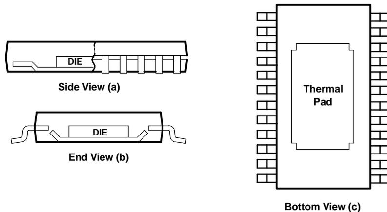
**Figure 36. Views of Thermally Enhanced PWP Package**
