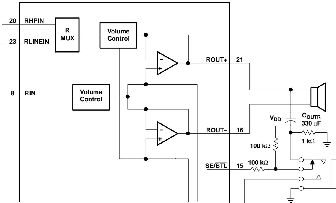
Figure 42. TPA0312 Resistor Divider Network Circuit
