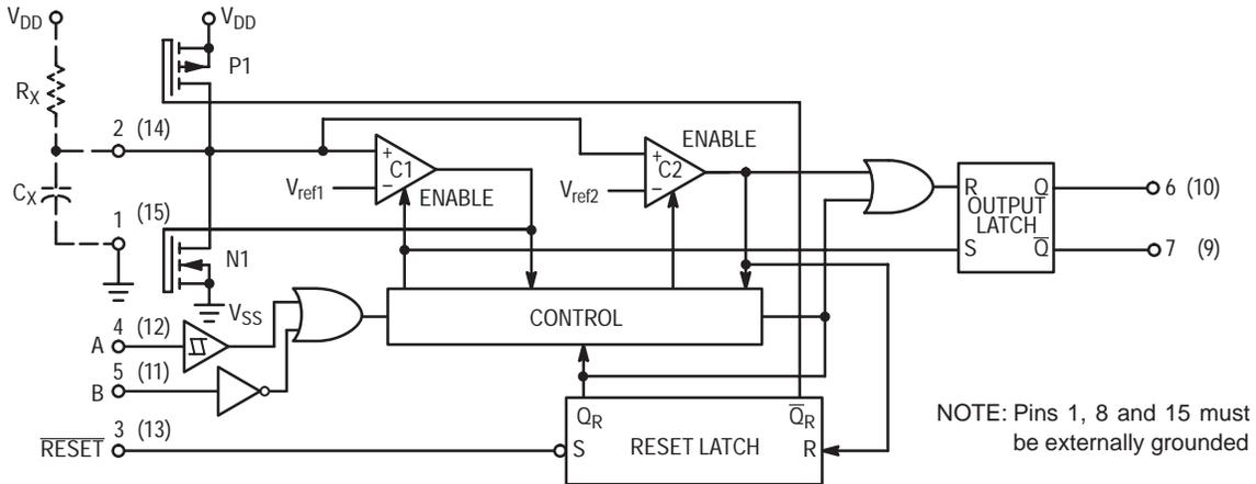
**Figure 1. Logic Diagram
