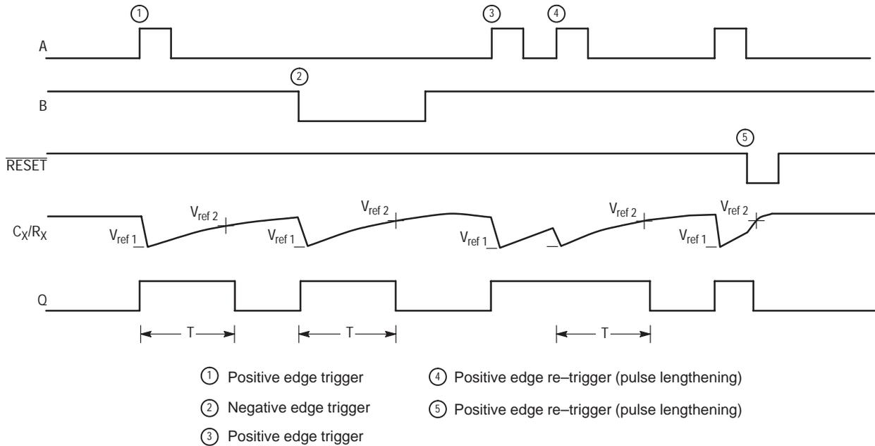
Figure 10. Timing Operation
