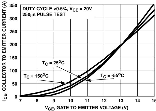
FIGURE 13. TRANSFER CHARACTERISTIC
