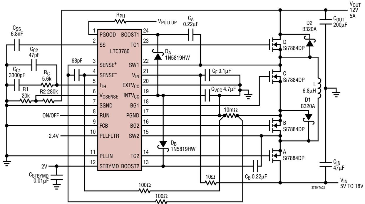
Figure 13. LTC3780 12V/5A, Buck-Boost Regulator
