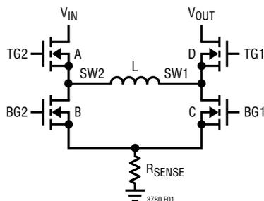
Figure 1. Simplified Diagram of the Output Switches
