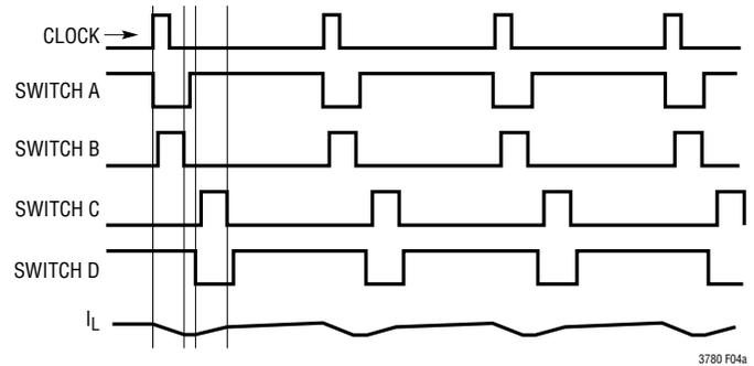
(4a) Buck-Boost Mode ( $V_{IN} \geq V_{OUT}$ )
