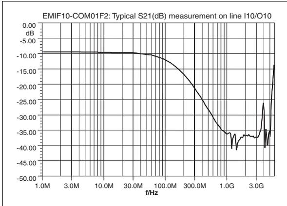
Note: Spikes at high frequencies are induced by the PCB layout
