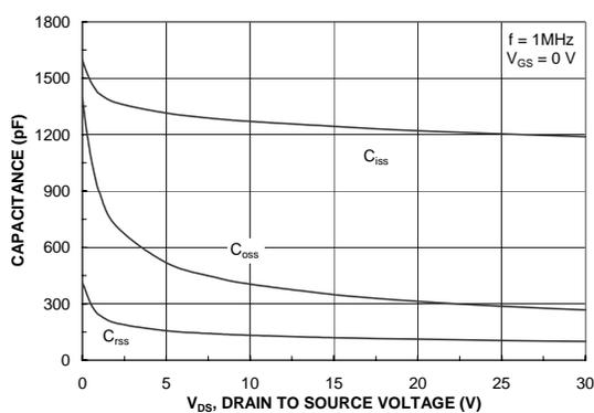
**Figure 8. Capacitance Characteristics.**
