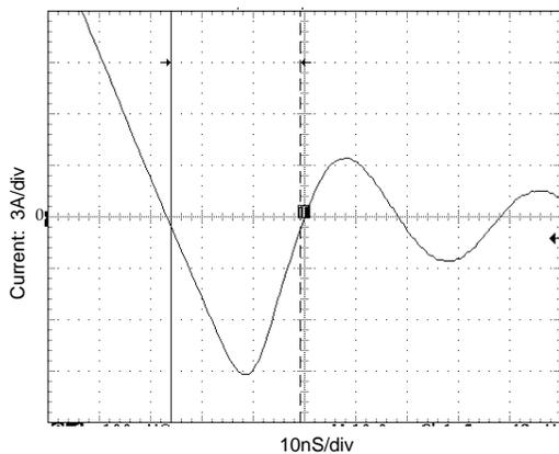
**Figure 13. Non-SyncFET (FDS6680) body diode reverse recovery characteristic.**
