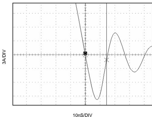
**Figure 12. FDS6680AS SyncFET body diode reverse recovery characteristic.**
