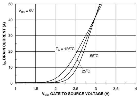
Figure 5. Transfer Characteristics.
