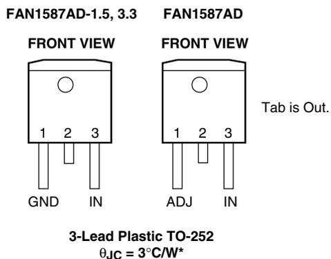
\*With package soldered to 0.5 square inch copper area over backside ground plane or internal power plane,  $\theta_{JA}$  can vary from  $30^{\circ}\text{C/W}$  to more than  $40^{\circ}\text{C/W}$ . Other mounting techniques can provide a thermal resistance lower than  $30^{\circ}\text{C/W}$ .
