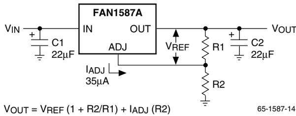
$$V_{OUT} = V_{REF} (1 + R2/R1) + I_{ADJ} (R2)$$
