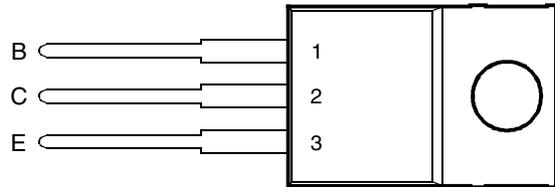
Pin 2 is in electrical contact with the mounting base.
