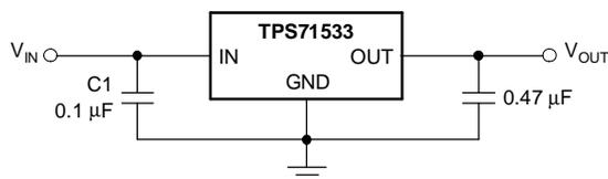
**Figure 13. Typical Application Circuit (Fixed Voltage Version)**
