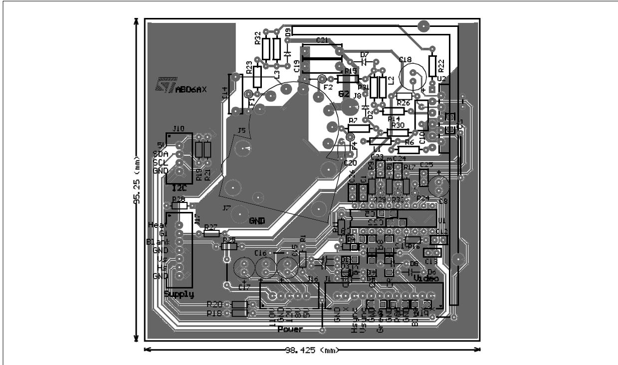
Figure 13. Amplifier and Preamp Output. Trace Routing (detail)
