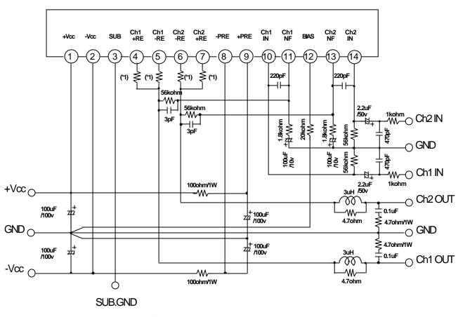
(\*1)Metal Plate Cement Resistor 0.22ohm+10%(5W)
