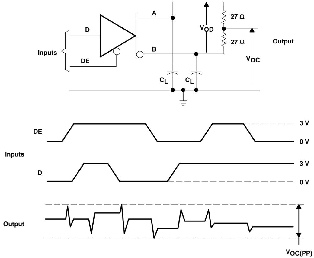
NOTES: A. Resistance values are in ohms and are 1% tolerance.
