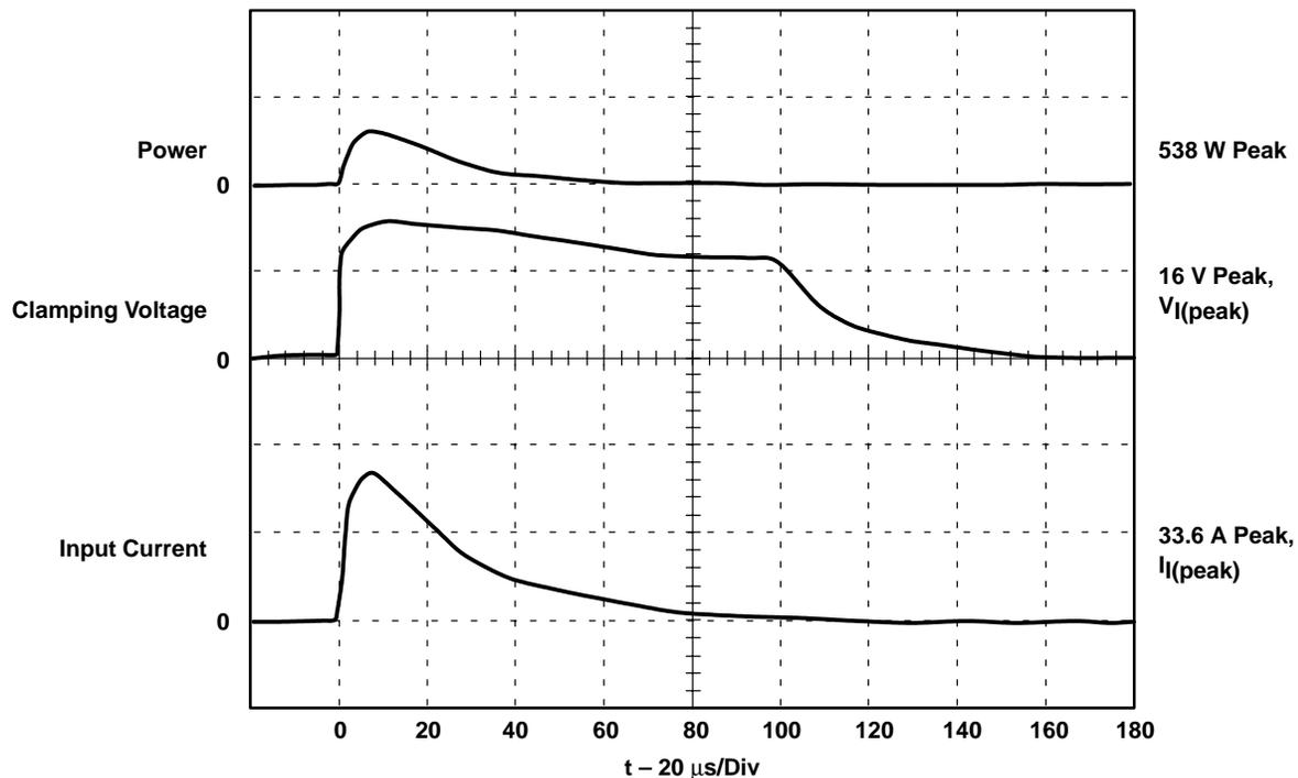
**Figure 17. Typical Surge Waveform Measured At Terminals 5 and 7**
