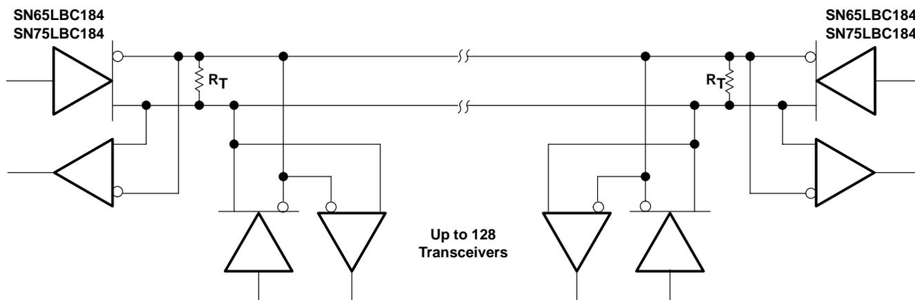
NOTE A: The line should be terminated at both ends in its characteristic impedance ( $R_T = Z_0$ ). Stub lengths off the main line should be kept as short as possible.
