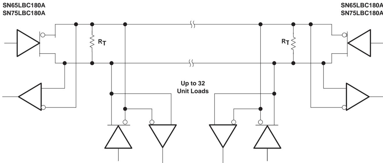
NOTE A: The line should be terminated at both ends in its characteristic impedance ( $R_T = Z_0$ ). Stub lengths off the main line should be kept as short as possible. One SN65LBC180A typically represents less than one unit load.
