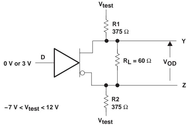
**Figure 2. Driver  $V_{OD}$**
