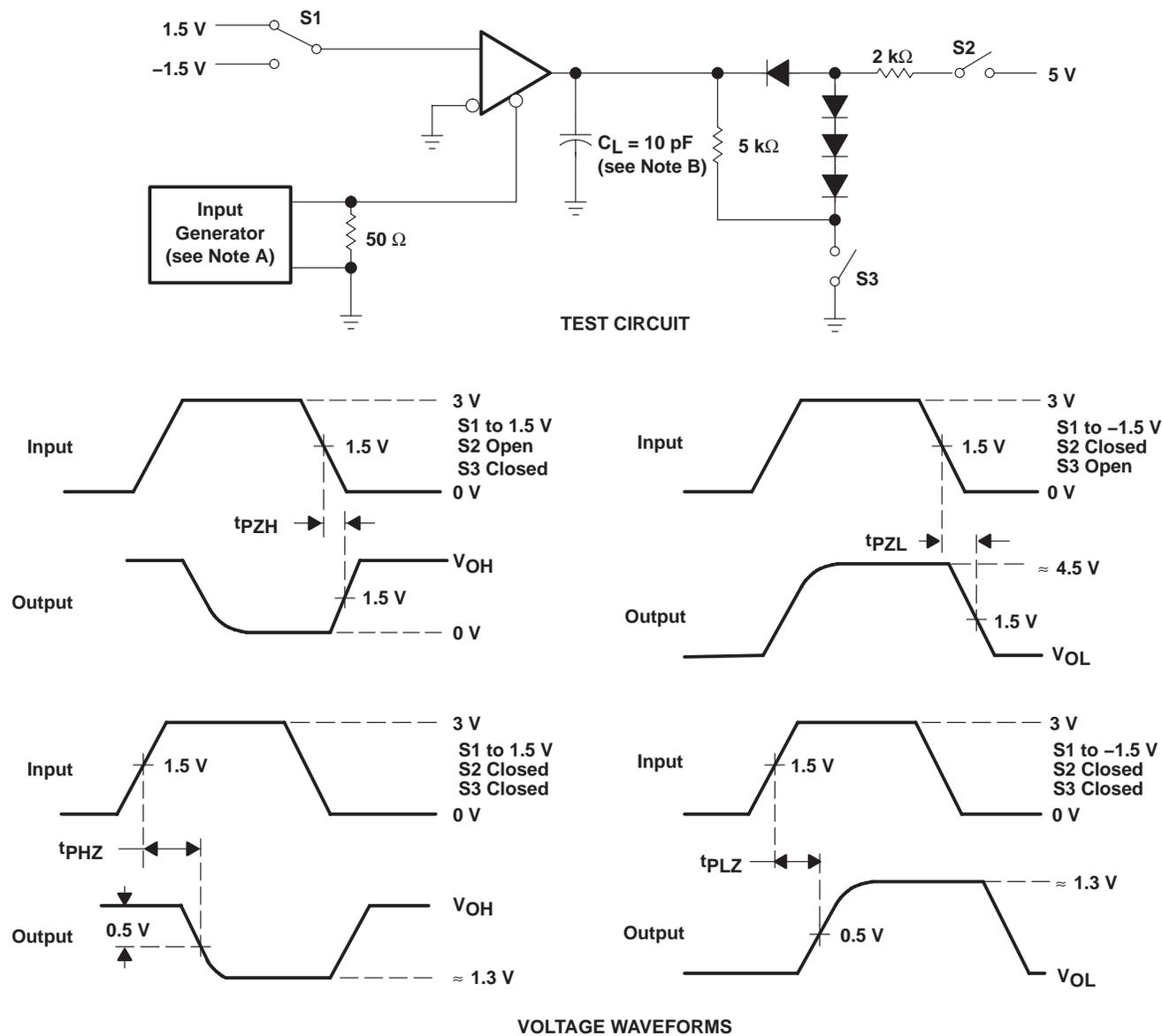
NOTES: A. The input pulse is supplied by a generator having the following characteristics: PRR ≤ 1 MHz, 50% duty cycle, tr ≤ 6 ns, tf ≤ 6 ns, ZO = 50 Ω.
