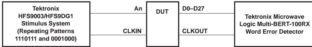
CLKIN is advanced or delayed with respect to data until errors are observed at the receiver outputs. The magnitude of the advance or delay is  $t_{RSKM}$ .
