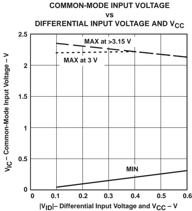
Figure 3. Recommended V<sub>IC</sub> Versus V<sub>ID</sub> and V<sub>CC</sub>
