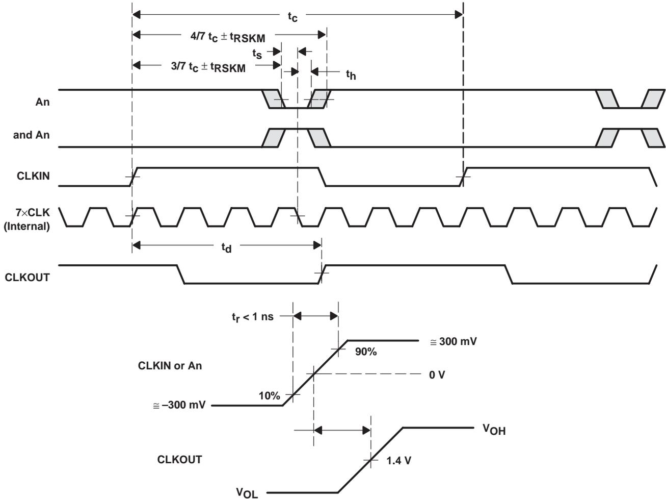
Figure 6. Receiver Input Skew Margin and  $t_d$  Definitions
