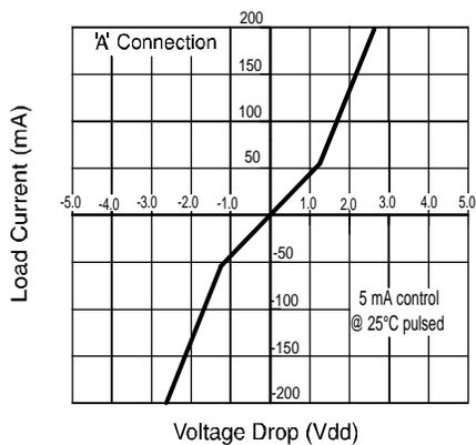
Figure 3. Linearity Characteristics
