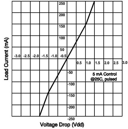
Figure 2. Linearity Characteristics
