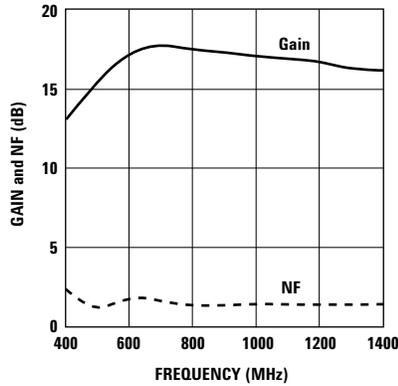
Figure 16. Gain and Noise Figure vs Frequency.
