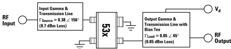
Figure 1. Block Diagram of 1.9 GHz Test Fixture.
