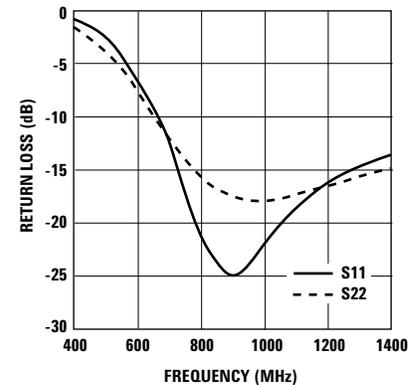
Figure 20. Input and Output return loss at 900 MHz.
