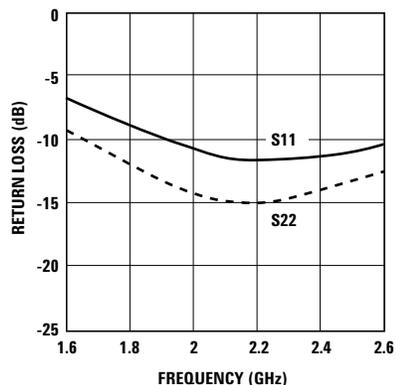
**Figure 12. Input and Output return loss vs Frequency.**
