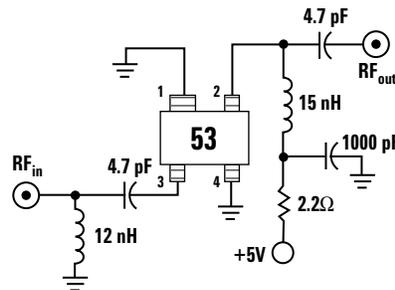
Figure 18. Schematic for 900 MHz LNA design.
