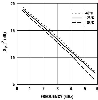
Figure 5.  $|S_{21}|^2$  vs. Frequency and Temperature.
