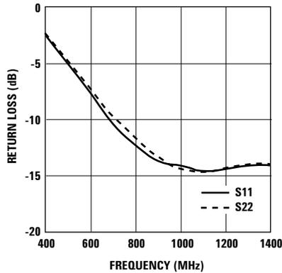
Figure 17. Input and Output return loss vs Frequency.
