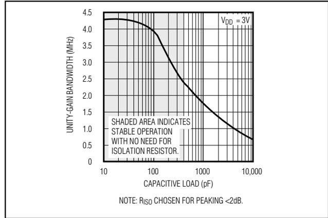
Figure 8. MAX4250-4254 Unity-Gain Bandwidth vs. Capacitive Load
