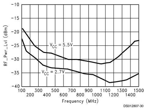
**Oscillator Input Sensitivity vs Frequency**
