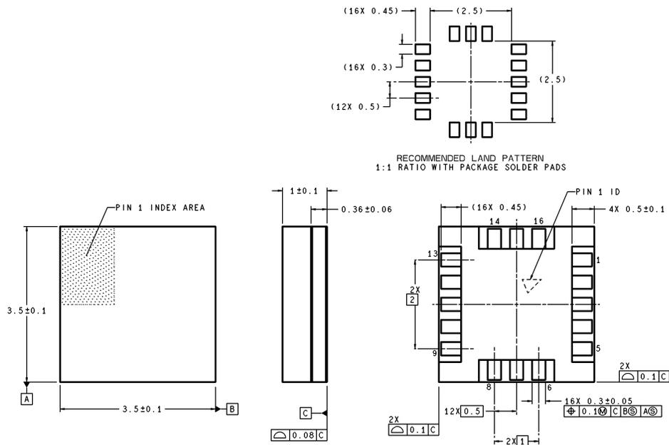
DIMENSIONS ARE IN MILLIMETERS
