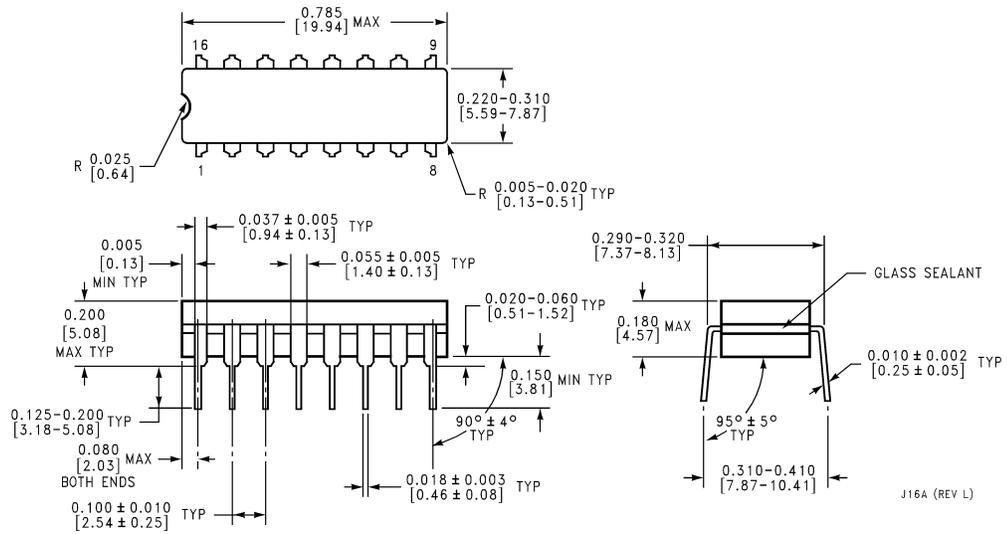
**16-Lead Ceramic Dual-in-Line Package**
