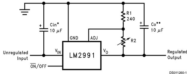
$$V_{OUT} = V_{REF} (1 + R2/R1)$$
