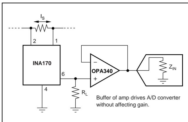
FIGURE 2. Buffering Output to Drive A/D Converter.
