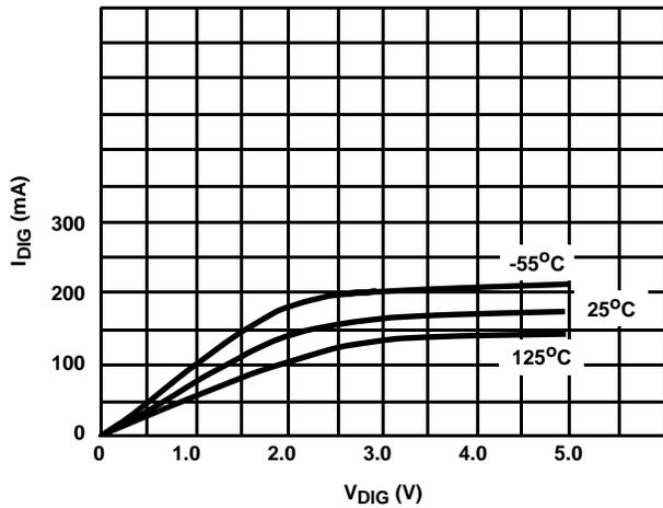
FIGURE 7. COMMON CATHODE DIGIT DRIVER  $I_{DIG}$  vs  $V_{DIG}$
