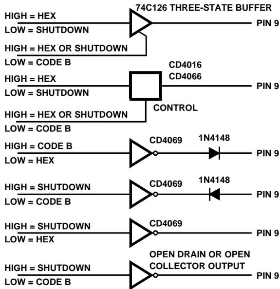
FIGURE 17. ICM7228C/D PIN 9 DRIVE CIRCUITS
