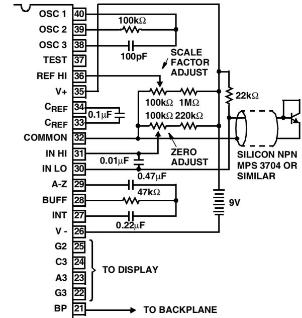
A silicon diode-connected transistor has a temperature coefficient of about  $-2\text{mV}/^\circ\text{C}$ . Calibration is achieved by placing the sensing transistor in ice water and adjusting the zeroing potentiometer for a 000.0 reading. The sensor should then be placed in boiling water and the scale-factor potentiometer adjusted for a 100.0 reading.
