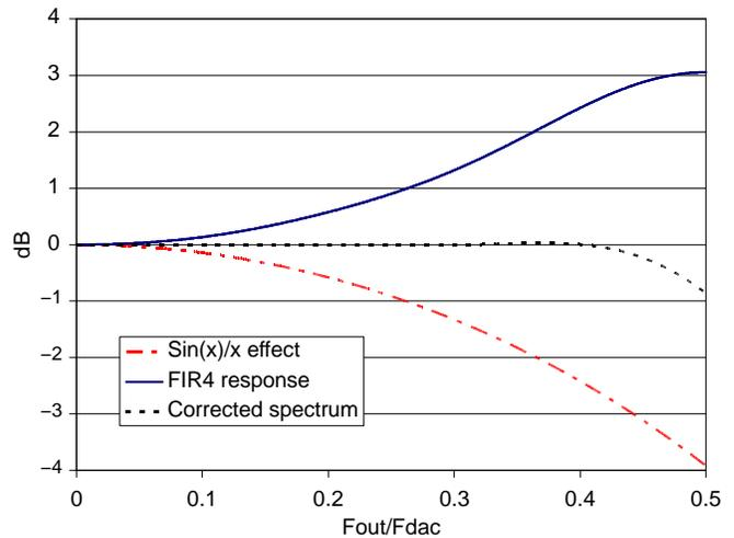
Figure 38. Magnitude Spectrum for Inverse Sinc Filter FIR4 (Versions 1 and 2)
