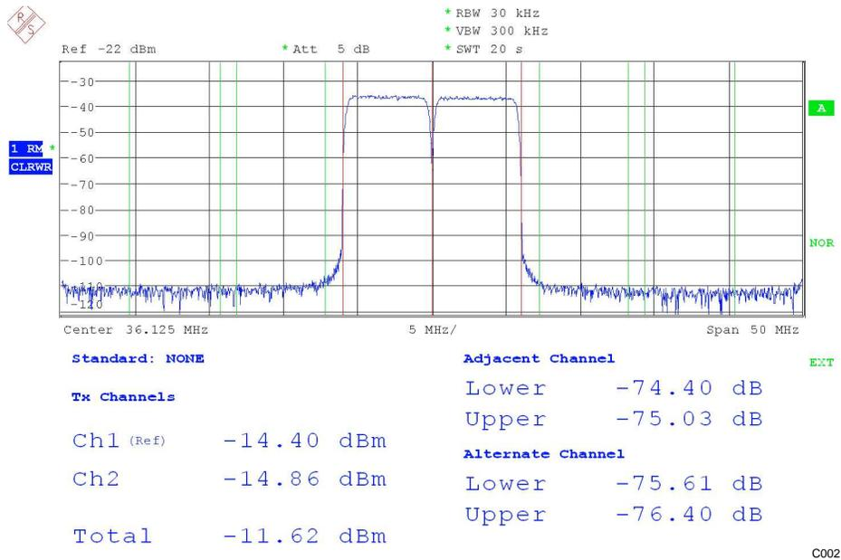
Figure 79. Two QAM256 Carriers With at 36-MHz IF
