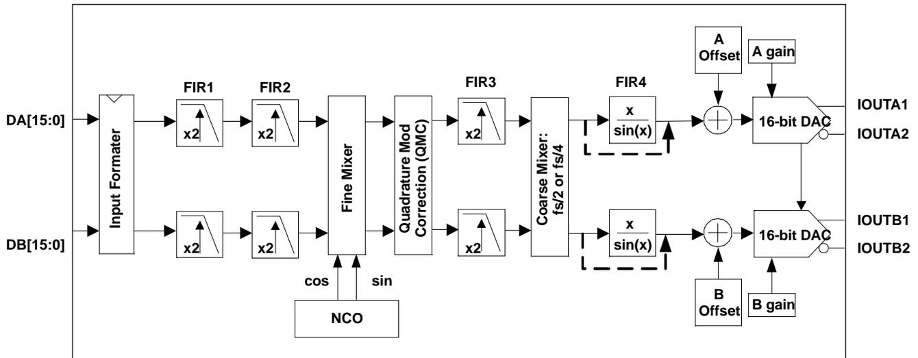
Figure 32. Block Diagram for X8 Mode
