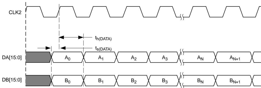
Figure 45. Dual Bus Mode Timing Diagram (PLL Mode)
