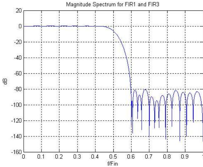
Figure 35. Magnitude Spectrum for FIR1 and FIR3
