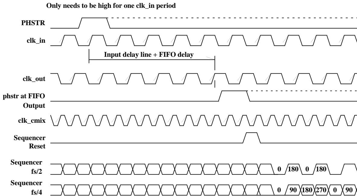
Figure 54. CMIX Reset Synchronization Timing
