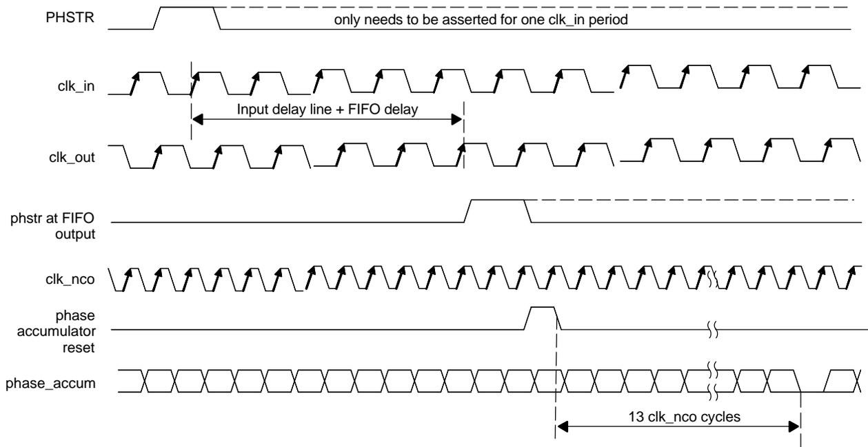
**Figure 52. NCO Phase Accumulator Reset Synchronization Timing**
