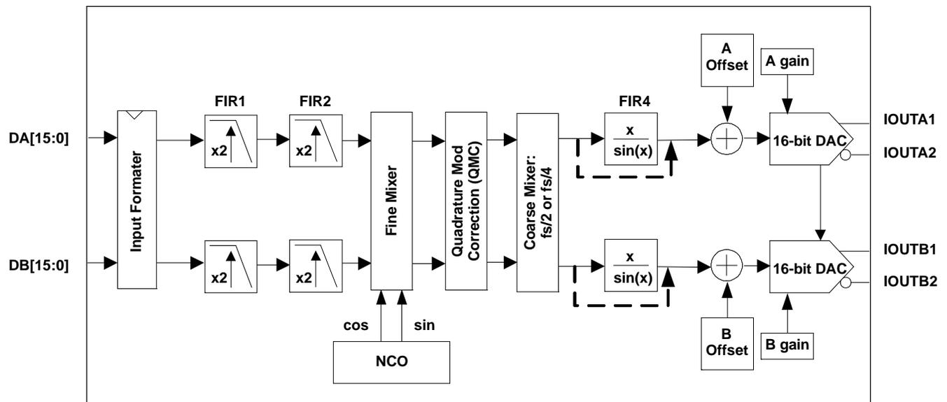
A. FMIX or QMC block cannot be enabled with CMIX block.
