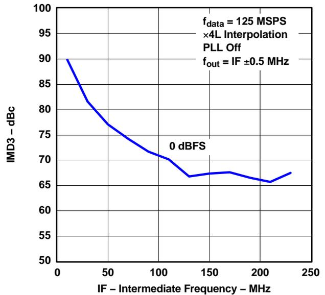
Figure 8. Two Tone IMD vs Intermediate Frequency
