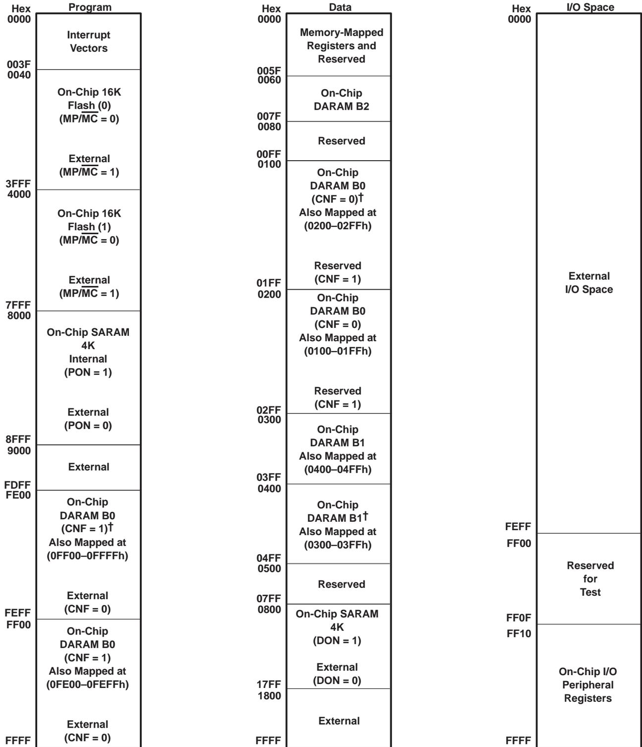
† DARAM blocks B0 and B1 are 256 × 16 words each; however, these memory blocks are mapped to dual address ranges within the 'F206 memory map. For more details, see the last paragraph in the memory section.
