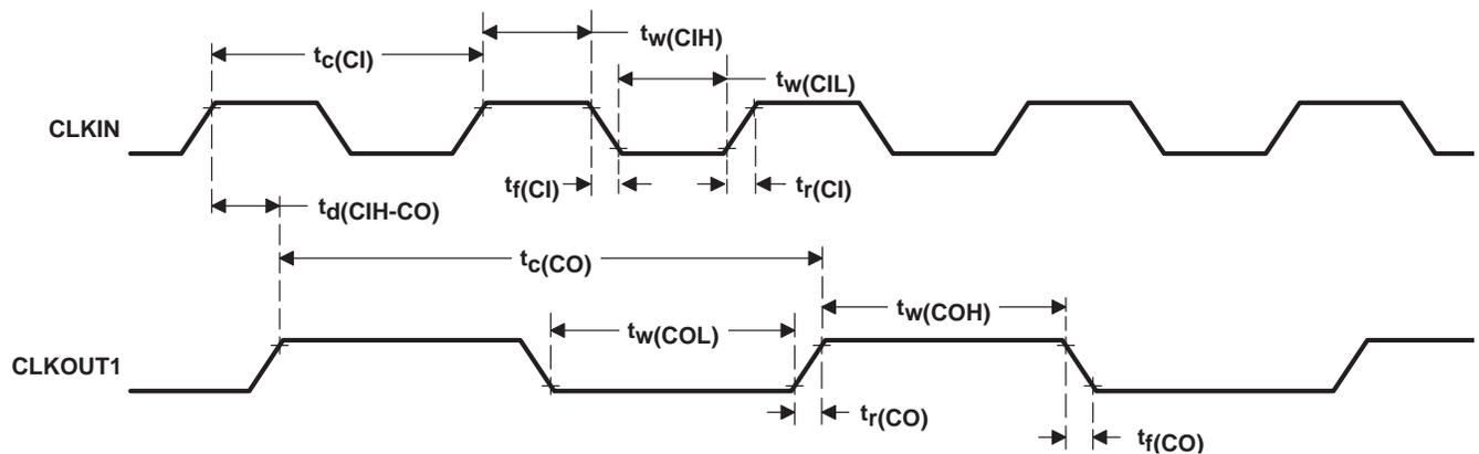
Figure 7. CLKIN-to-CLKOUT1 Timing Without PLL (using ÷2 clock option)
