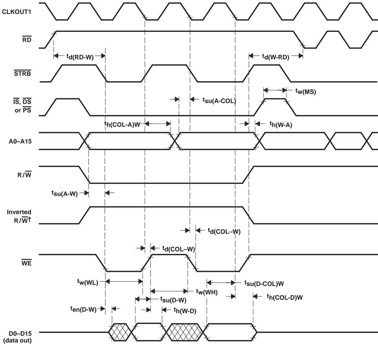
† If the FRDN bit in the PMST register (FFE4h) is a 1, then the signal issued from the  $\overline{RD}$  pin (pin 45) is an inverted R/ $\overline{W}$  signal (or fast  $\overline{RD}$ ) replacing the RD signal.
