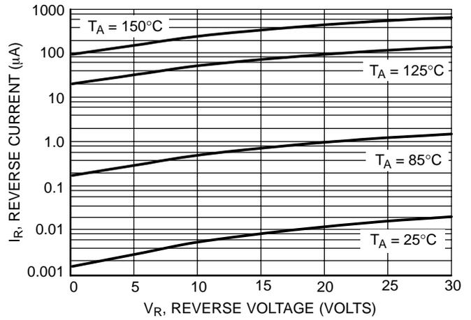
**Figure 3. Leakage Current**
