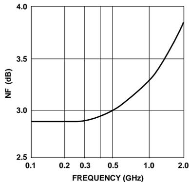
**Figure 4. Noise Figure vs. Frequency,  $I_d = 29 \text{ mA}$ .**
