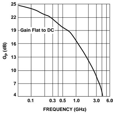
**Figure 1. Power Gain vs. Frequency,  $I_d = 29 \text{ mA}$ .**
