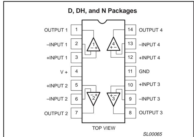
Figure 1. Pin configuration.
