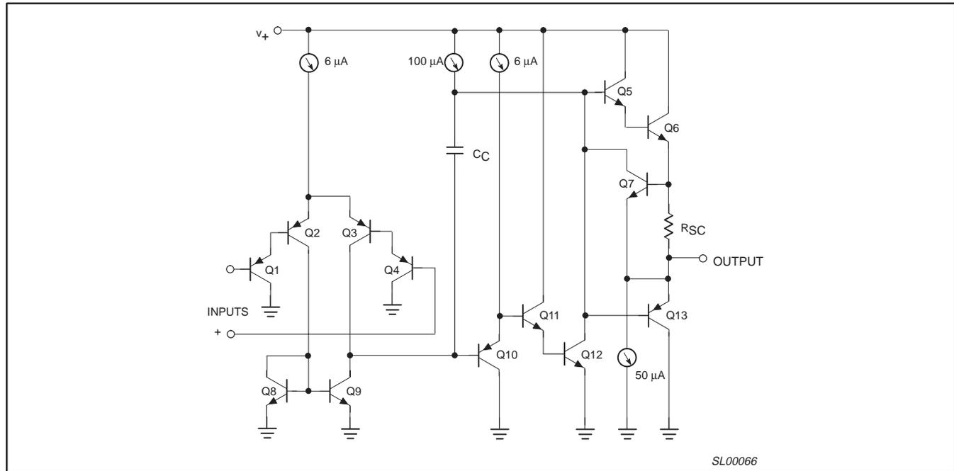
Figure 2. Equivalent circuit.
