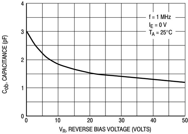
Figure 10. Output Capacitance
