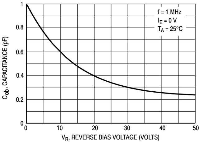
Figure 15. Output Capacitance
