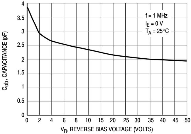
Figure 20. Output Capacitance
