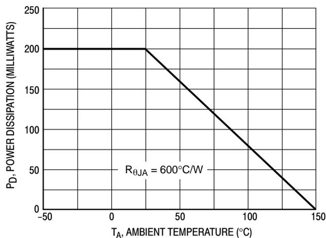
Figure 1. Derating Curve
