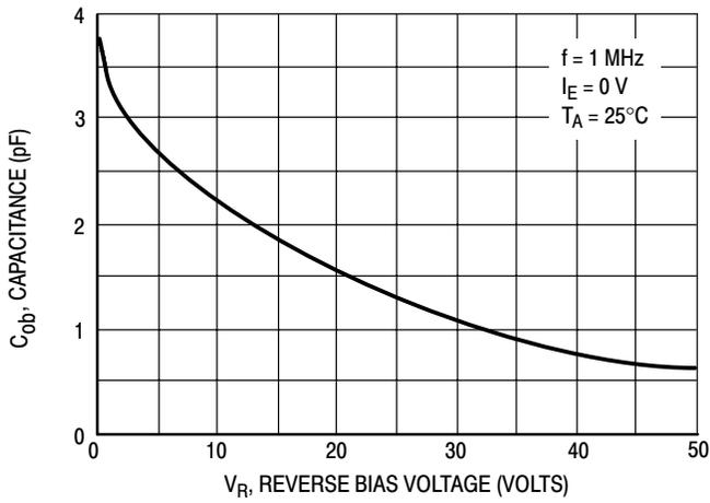
Figure 5. Output Capacitance
