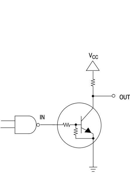
Figure 24. Open Collector Inverter: Inverts the Input Signal
