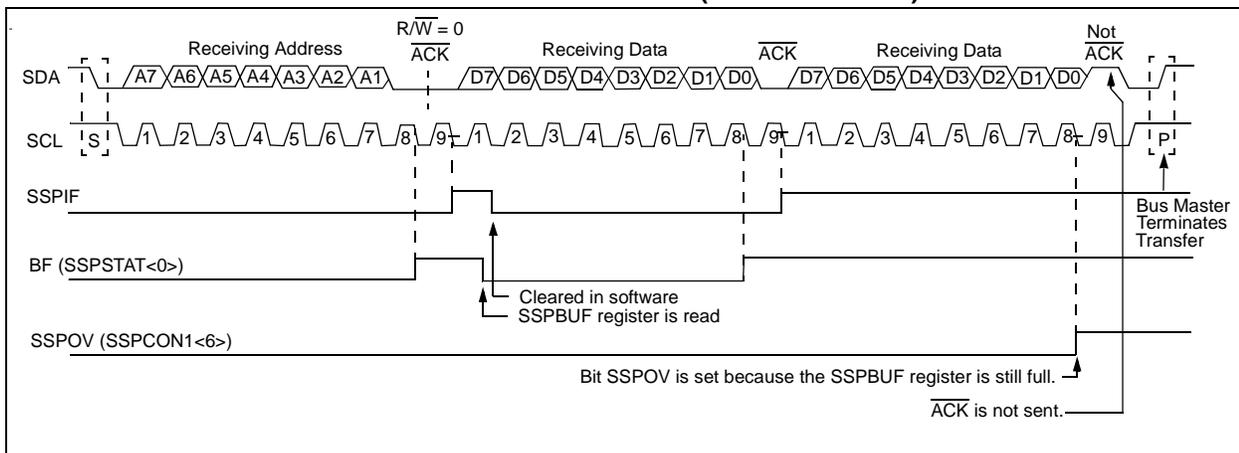
**FIGURE 15-13: I<sup>2</sup>C WAVEFORMS FOR TRANSMISSION (7-BIT ADDRESS)**
