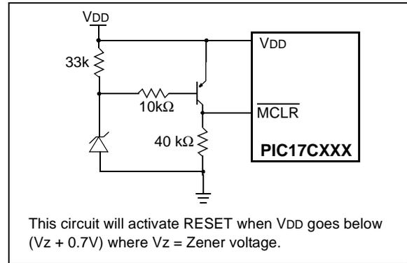
**FIGURE 5-9: EXTERNAL BROWN-OUT PROTECTION CIRCUIT 2**
