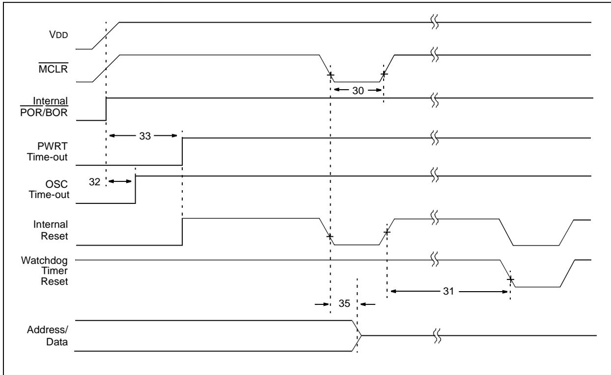
**TABLE 20-3: RESET, WATCHDOG TIMER, OSCILLATOR START-UP TIMER, POWER-UP TIMER, AND BROWN-OUT RESET REQUIREMENTS**
