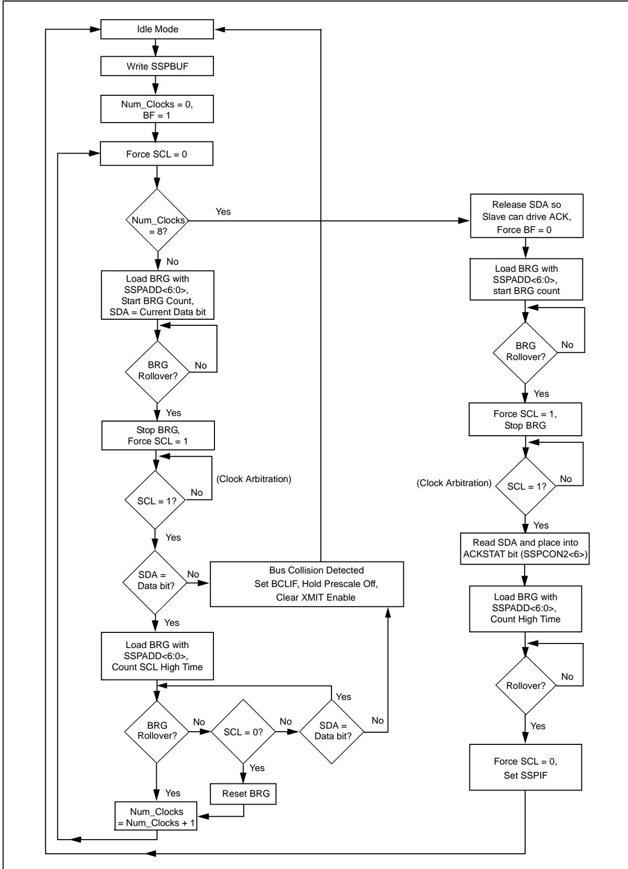
**FIGURE 15-26: I<sup>2</sup>C MASTER MODE TIMING (TRANSMISSION, 7 OR 10-BIT ADDRESS)**
