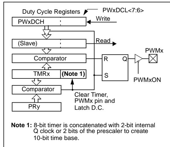
**FIGURE 13-4: PWM OUTPUT (NOT BUFFERED)**
