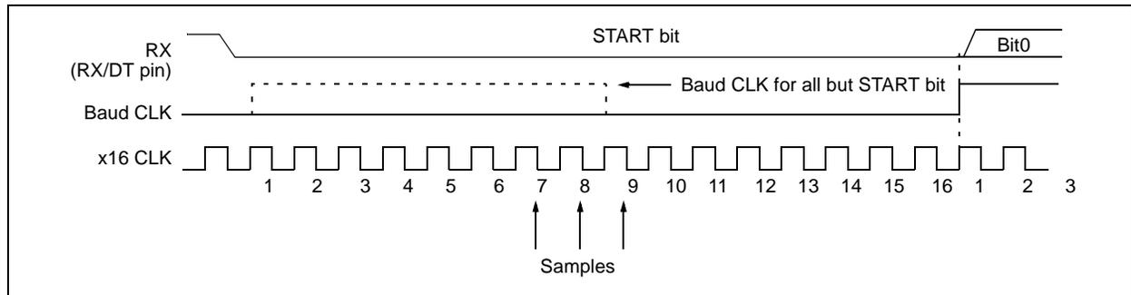
**FIGURE 14-6: START BIT DETECT**
