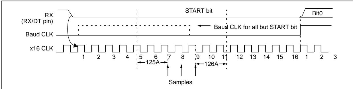
**TABLE 20-17: USART ASYNCHRONOUS RECEIVE SAMPLING REQUIREMENTS**
