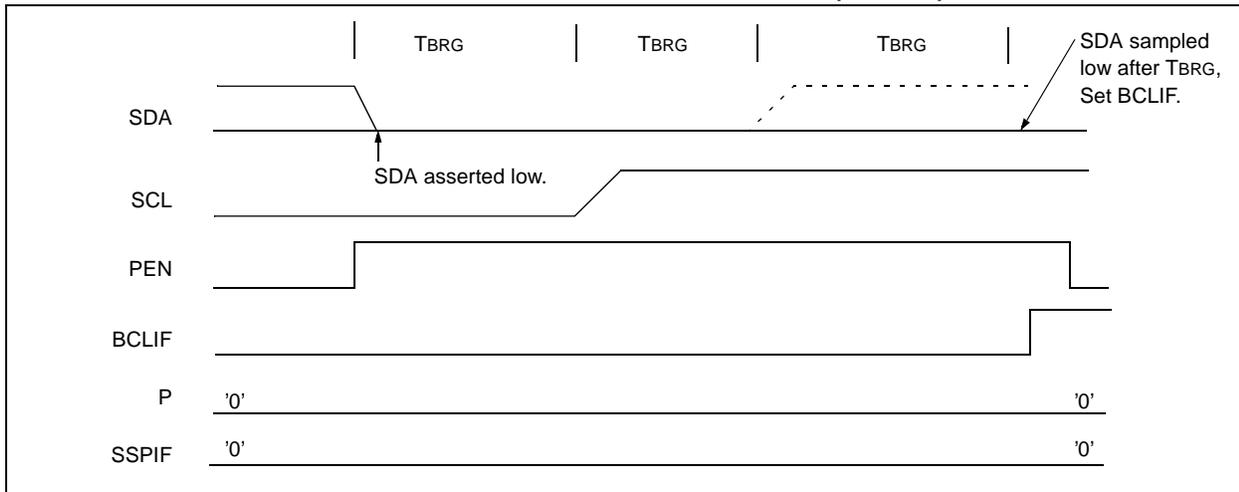
**FIGURE 15-41: BUS COLLISION DURING A STOP CONDITION (CASE 2)**
