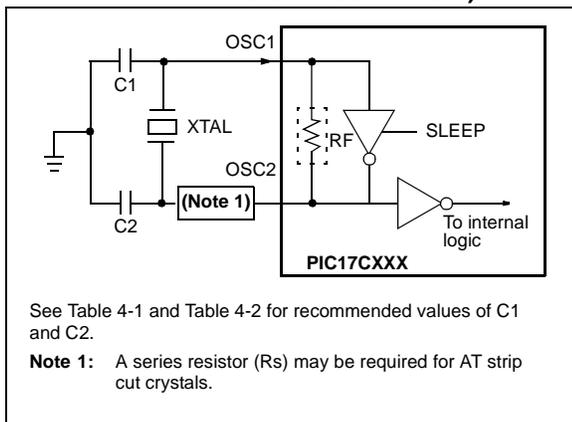
**FIGURE 4-3: CRYSTAL OPERATION, OVERTONE CRYSTALS (XT OSC CONFIGURATION)**
