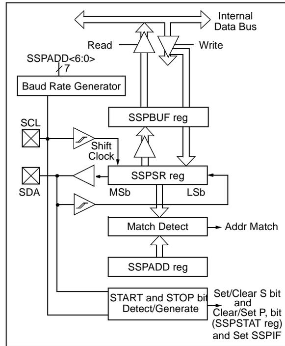
Two pins are used for data transfer. These are the SCL pin, which is the clock and the SDA pin, which is the data. The SDA and SCL pins are automatically configured when the I<sup>2</sup>C mode is enabled. The SSP module functions are enabled by setting SSP Enable bit SSPEN (SSPCON1<5>).
