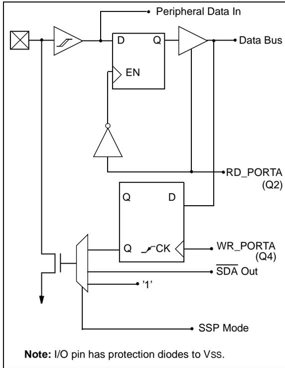
**FIGURE 10-4: RA4 AND RA5 BLOCK DIAGRAM**
