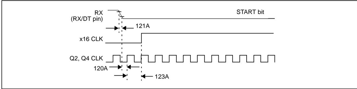
**TABLE 20-16: USART ASYNCHRONOUS MODE START BIT DETECT REQUIREMENTS**
