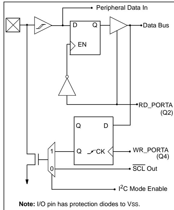
**FIGURE 10-3: RA3 BLOCK DIAGRAM**
