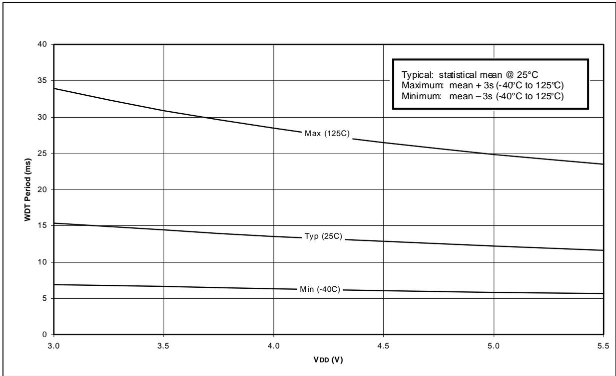
**FIGURE 21-16: TYPICAL WDT PERIOD vs. V<sub>DD</sub> OVER TEMPERATURE (-40°C TO +125°C)**
