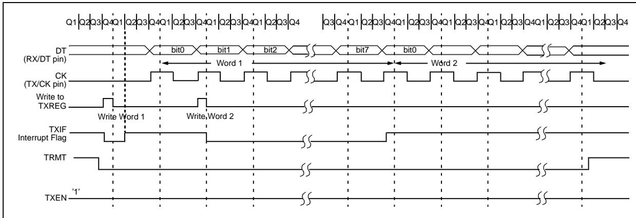
**FIGURE 14-9: SYNCHRONOUS TRANSMISSION (THROUGH TXEN)**
