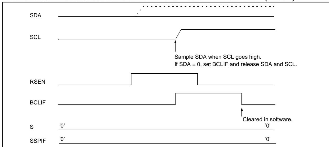
**FIGURE 15-39: BUS COLLISION DURING REPEATED START CONDITION (CASE 2)**
