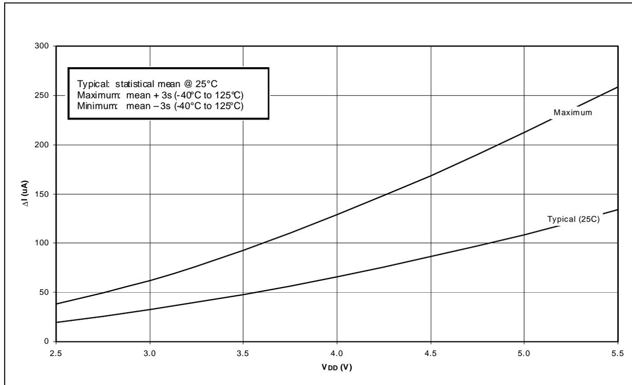
**FIGURE 21-15: TYPICAL, MINIMUM AND MAXIMUM WDT PERIOD vs. V<sub>DD</sub> (-40°C TO +125°C)**
