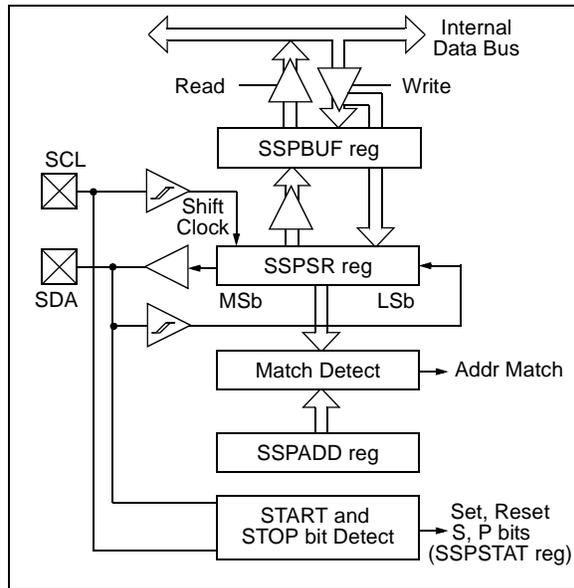
**FIGURE 15-11: I<sup>2</sup>C MASTER MODE BLOCK DIAGRAM**
