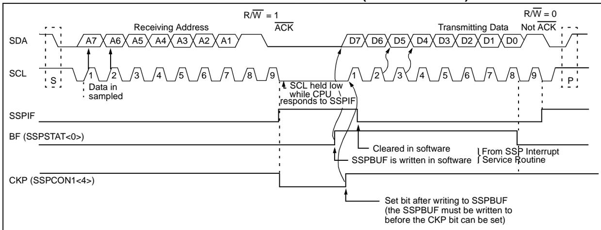
**FIGURE 15-14: I<sup>2</sup>C SLAVE-TRANSMITTER (10-BIT ADDRESS)**
