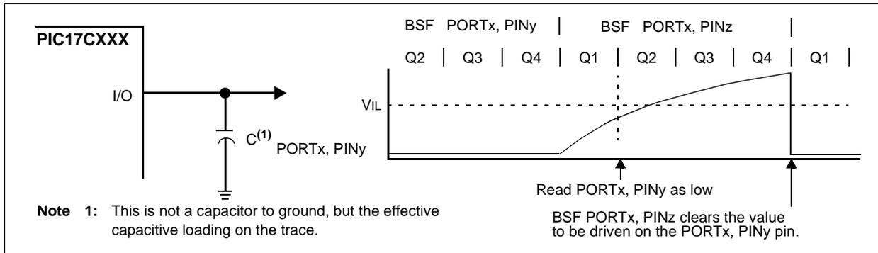
**Note 1:** This is not a capacitor to ground, but the effective capacitive loading on the trace.
