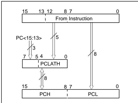
Using Figure 7-7, the operations of the PC and PCLATH for different instructions are as follows:
