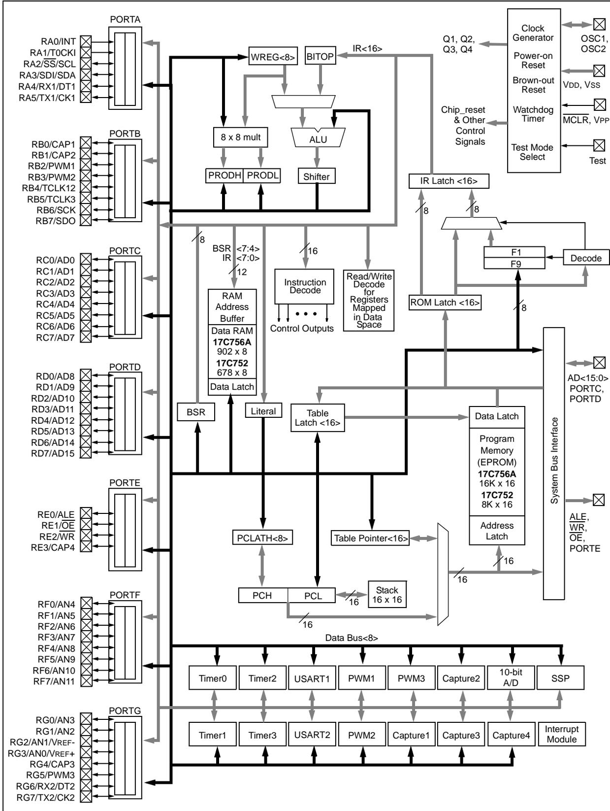
**FIGURE 3-2: PIC17C762/766 BLOCK DIAGRAM**
