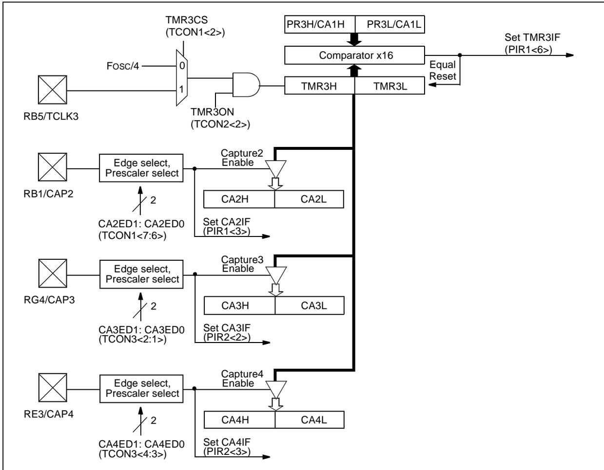
This mode (3 Capture, 1 Period) is selected if control bit CA1/ $\overline{\text{PR3}}$  is clear. In this mode, the Capture1 register, consisting of high byte (PR3H/CA1H) and low byte (PR3L/CA1L), is configured as the period control register for TMR3. Capture1 is disabled in this mode and the corresponding interrupt bit, CA1IF, is never set. TMR3 increments until it equals the value in the period register and then resets to 0000h on the next timer clock.
