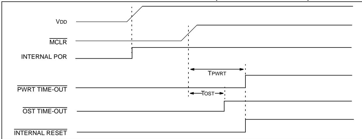
**FIGURE 5-7: SLOW RISE TIME ( $\overline{\text{MCLR}}$  TIED TO  $V_{DD}$ )**
