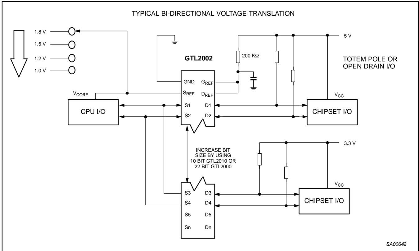
Figure 1. Bi-directional translation to multiple higher voltage levels such as an I<sup>2</sup>C bus application
