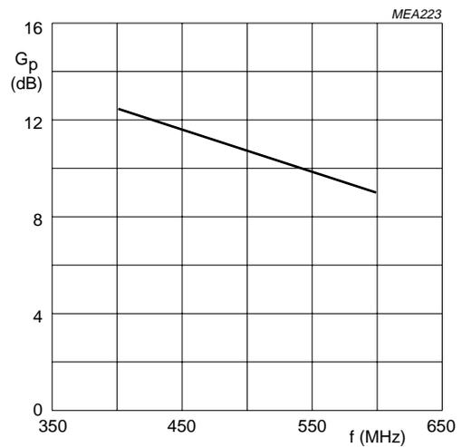
Class-B operation;  $V_{CE} = 7.5$  V;  $P_L = 1.2$  W.
