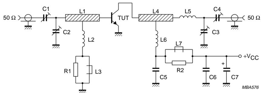
Fig.6 Class-B test circuit at  $f = 470$  MHz.
