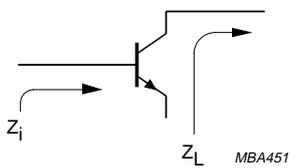
Fig. 10 Definition of transistor impedance.
