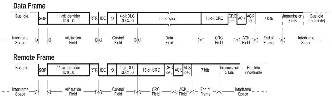
A message in the CAN standard frame format begins with the "Start Of Frame (SOF)", this is followed by the "Arbitration field" which consist of the identifier and the "Remote Transmission Request (RTR)" bit used to distinguish between the data frame and the data request frame called remote frame. The following "Control field" contains the "Identifier Extension (IDE)" bit and the "Data Length Code (DLC)" used to indicate the
