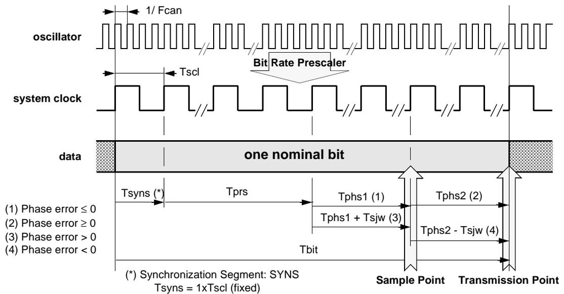
Tbit calculation:  $T_{bit} = T_{sycl} + T_{prs} + T_{phs1} + T_{phs2}$
