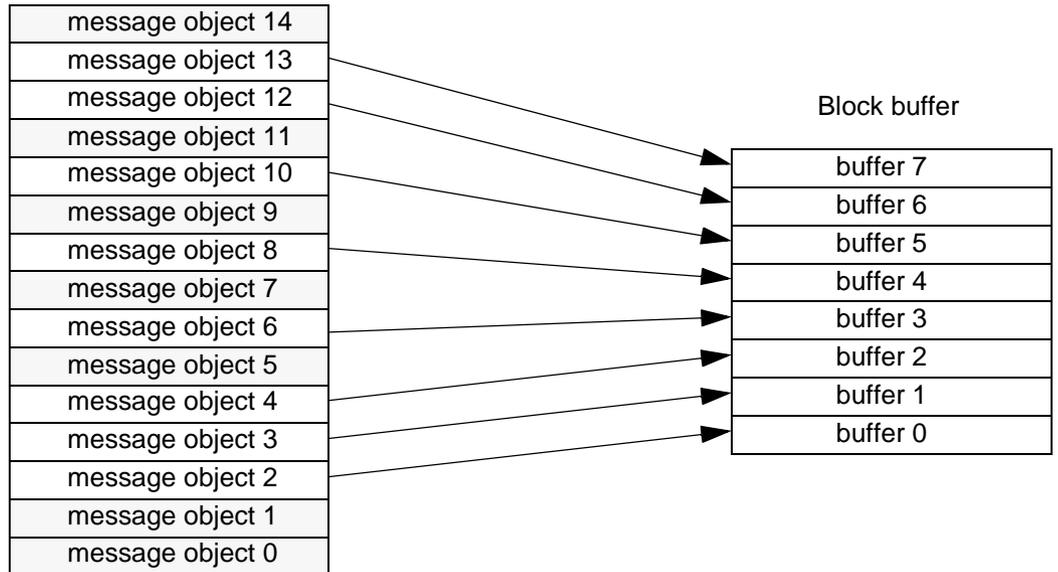
The same acceptance filter must be defined for each message objects of the buffer. When there is no mask on the identifier or the IDE, all messages are accepted.
