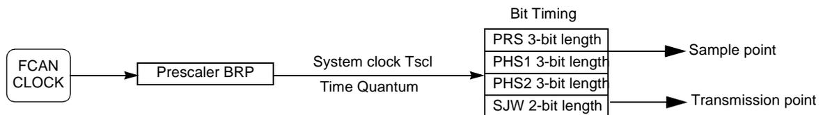
The baud rate selection is made by Tbit calculation:
