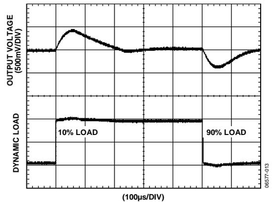
Figure 16. Typical Transient Load Response, 3 V Output, 10% to 90% Load Step
