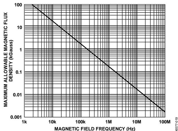
Figure 25. Maximum Allowable External Magnetic Flux Density
