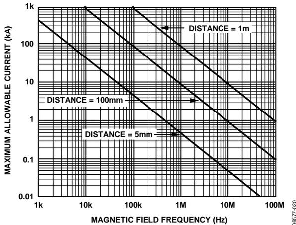
Figure 26. Maximum Allowable Current for Various Current-to-ADuM5401/ADuM5402/ADuM5403/ADuM5404 Spacings
