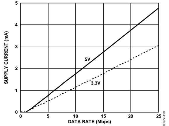
Figure 21. Typical  $I_{ISO(D)}$  Dynamic Supply Current per Input
