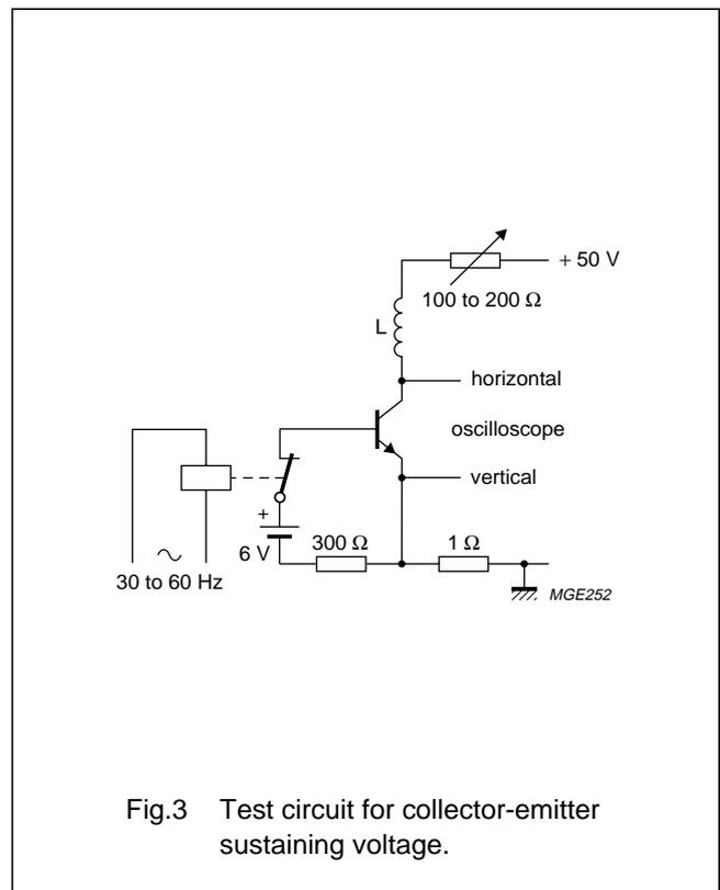
Silicon diffused power transistors
