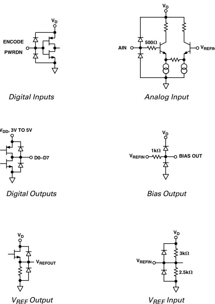
Figure 6. Equivalent Circuits
