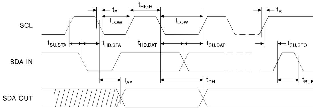
**Write Cycle Timing (SCL: Serial Clock, SDA: Serial Data I/O)**
