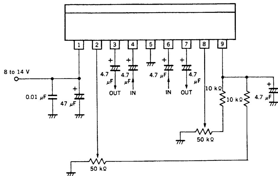
(2) To Balance The Two Attenuators
