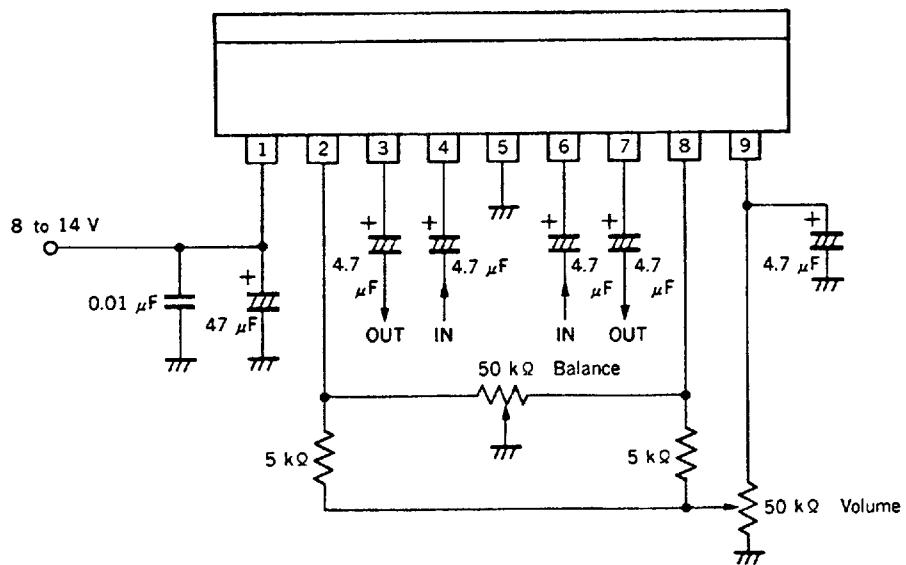
(3) To Control Both Attenuators Simultaneously
