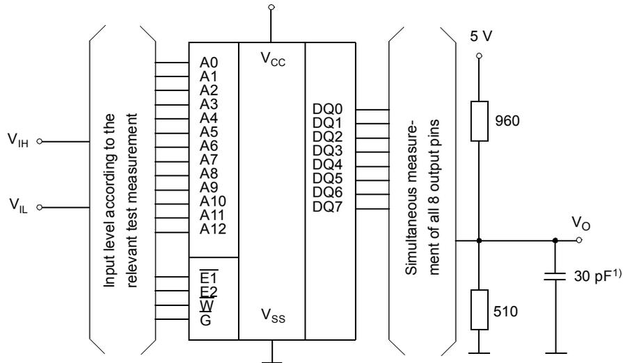
1) In measurement of  $t_{dis(E)}$ ,  $t_{dis(W)}$ ,  $t_{dis(G)}$  the capacitance is 5 pF.
