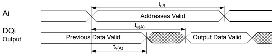
Read Cycle 2 (during Read cycle:  $\overline{W} = V_{IH}$ )
