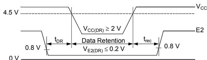
Chip Deselect to Data Retention Time  $t_{DR}$  : min 0 ns
