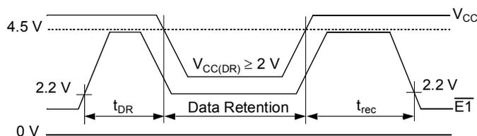
$$V_{E2(DR)} \geq V_{CC(DR)} - 0.2 \text{ V or } V_{E2(DR)} \leq 0.2 \text{ V}$$
