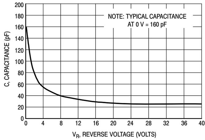
Figure 3. Typical Capacitance
