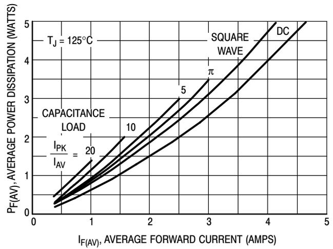
Figure 5. Power Dissipation
