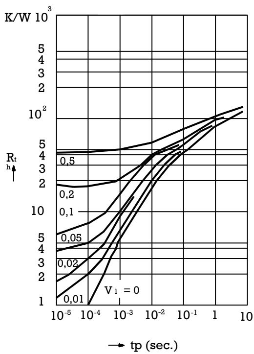
Pulse thermal resistance versus pulse duration. Valid provided that leads are kept at ambient temperature at a distance of 10 mm. from case.
