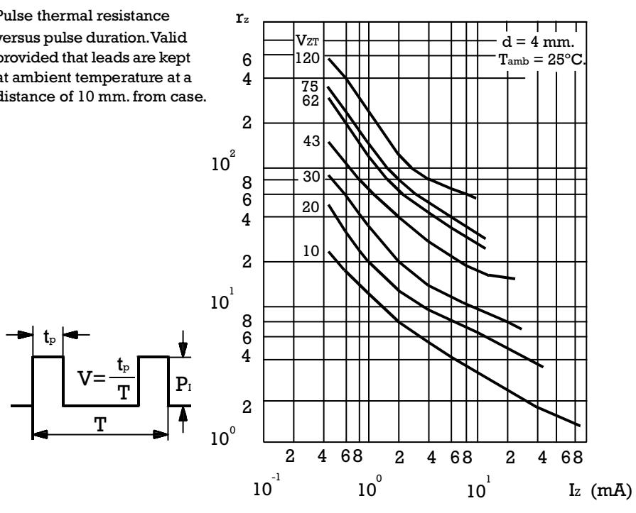
Differential resistance  $r_z$  vs. current  $I_z$  for several regulation voltages  $V_{ZT}$
