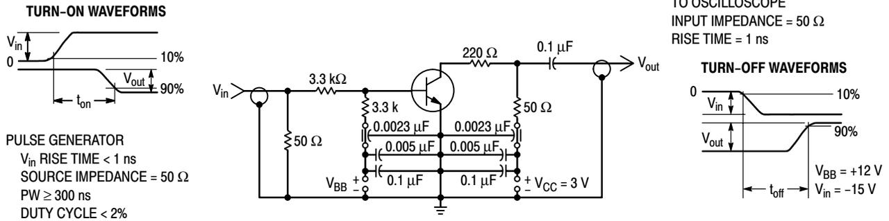
Figure 5. Turn-On and Turn-Off Time Test Circuit
