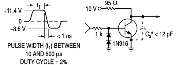
Figure 4.  $t_{off}$  Circuit – 100 mA
