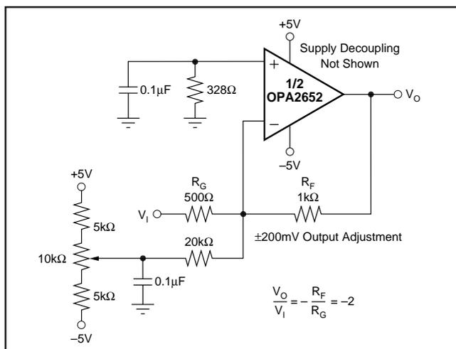
FIGURE 9. DC-Coupled, Inverting Gain of  $-2$ , with Offset Adjustment.
