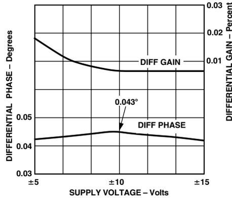
Figure 20. Differential Gain & Phase vs. Supply
