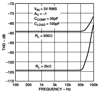
Figure 16. Total Harmonic Distortion (THD) vs. Frequency
