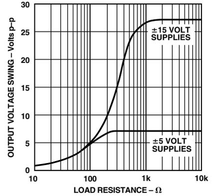
Figure 3. Output Voltage Swing vs. Resistive Load
