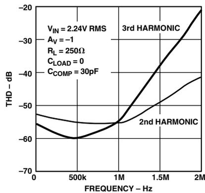
Figure 17. 2nd & 3rd Harmonic Distortion vs. Frequency
