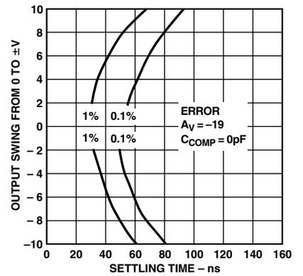
Figure 15. Output Swing & Error vs. Settling Time
