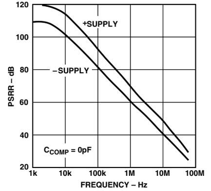
Figure 12. Power Supply Rejection Ratio (PSRR) vs. Frequency
