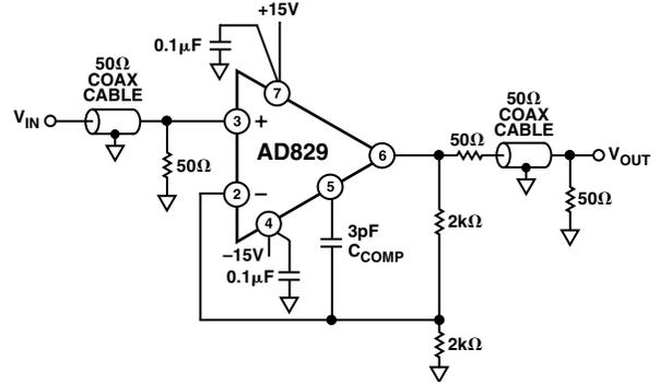
Figure 36. Noninverting Amplifier Connection Using Current Feedback Compensation
