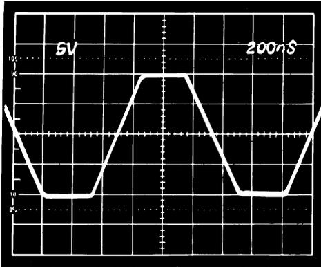
Figure 30. Large Signal Pulse Response of Inverting Amplifier Using Current Feedback Compensation.  $C_{COMP} = 15 \text{ pF}$ ,  $C_1 = 15 \text{ pF}$ ,  $R_F = 1 \text{ k}\Omega$ ,  $R_1 = 1 \text{ k}\Omega$
