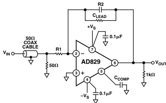
Figure 26. Inverting Amplifier Connection Using External Shunt Compensation
