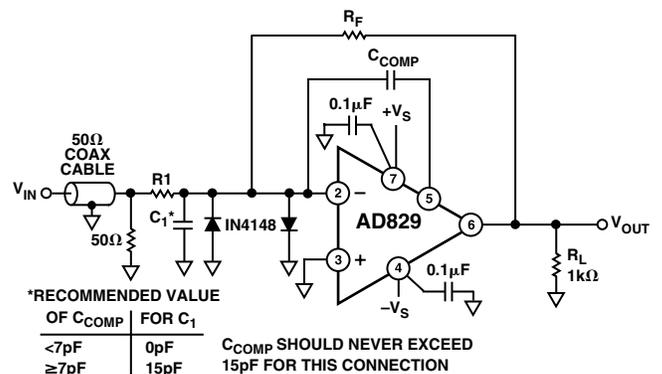
Figure 29. Inverting Amplifier Connection Using Current Feedback Compensation
