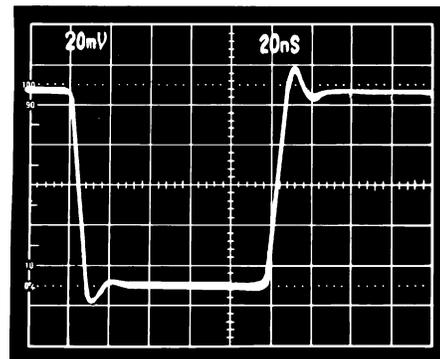
Figure 22c. Gain-of-2 Follower Small Signal Pulse Response
