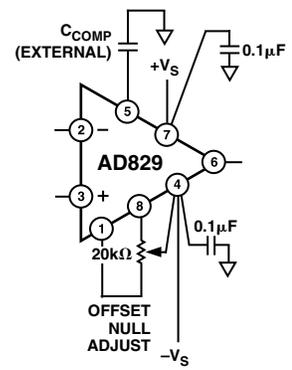
Figure 21. Offset Null and External Shunt Compensation Connections
