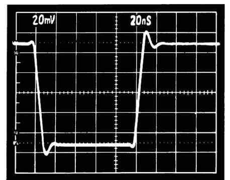
Figure 24c. Unity Gain Inverter Small Signal Pulse Response
