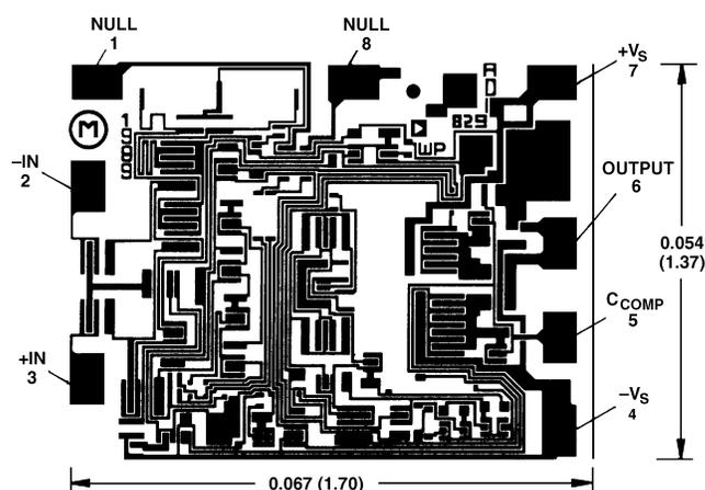
SUBSTRATE CONNECTED TO +V<sub>S</sub>
