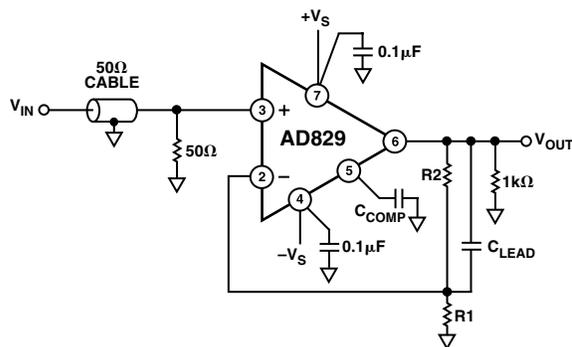
Figure 27. Noninverting Amplifier Connection Using External Shunt Compensation
