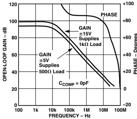
Figure 10. Open-Loop Gain & Phase Margin vs. Frequency
