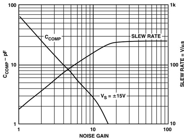
Figure 28. Value of C<sub>COMP</sub> & Slew Rate vs. Noise Gain
