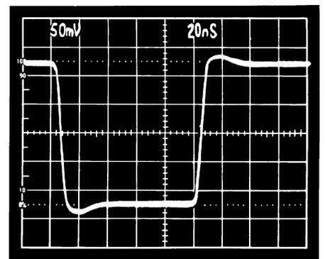
Figure 23c. Gain-of-20 Follower Small Signal Pulse Response
