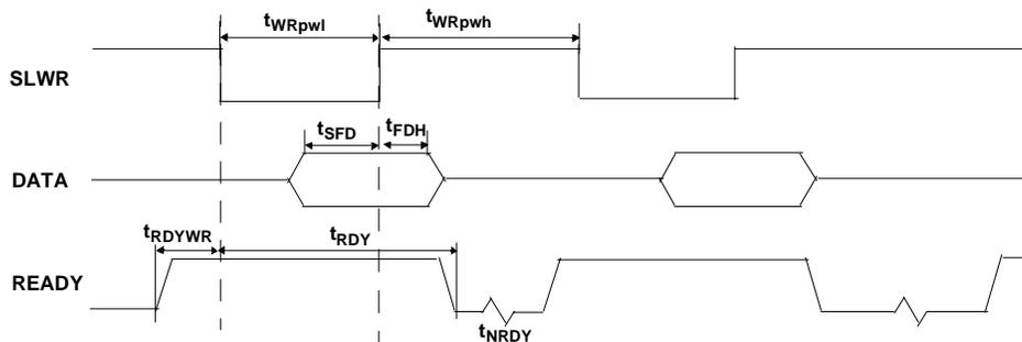
**Figure 11-4. Command Asynchronous Write Timing Diagram<sup>[12]</sup>**
