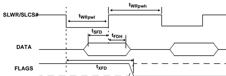
**Figure 11-10. Slave FIFO Asynchronous Write Timing Diagram<sup>[12]</sup>**
