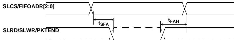
**Figure 11-12. Slave FIFO Asynchronous Address Timing Diagram<sup>[12]</sup>**
