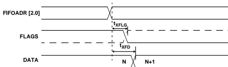
**Figure 11-13. Slave FIFO Address to Flags/Data Timing Diagram<sup>[11]</sup>**
