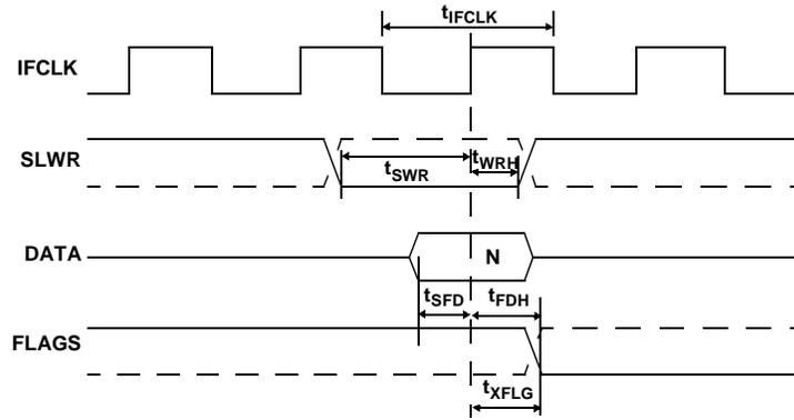
**Figure 11-6. Slave FIFO Synchronous Write Timing Diagram<sup>[12]</sup>**
