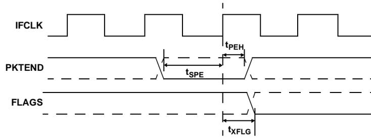
**Figure 11-7. Slave FIFO Synchronous Packet End Strobe Timing Diagram<sup>[12]</sup>**
