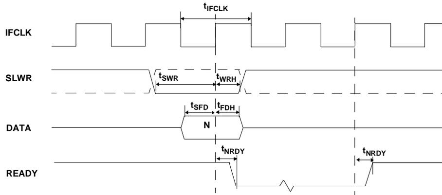
Figure 11-2. Command Synchronous Write Timing Diagram<sup>[12]</sup>
