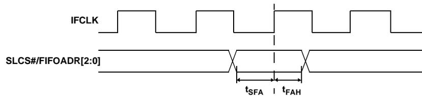
**Figure 11-8. Slave FIFO Synchronous Address Timing Diagram**
