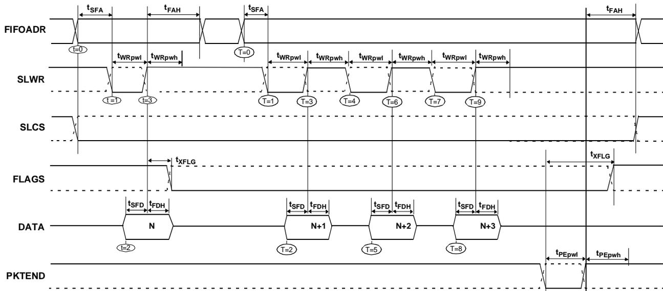
**Figure 11-20. Slave FIFO Asynchronous Write Sequence and Timing Diagram<sup>[12]</sup>**
