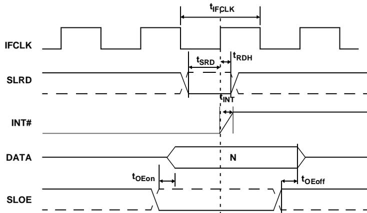
Figure 11-1. Command Synchronous Read Timing Diagram<sup>[12]</sup>
