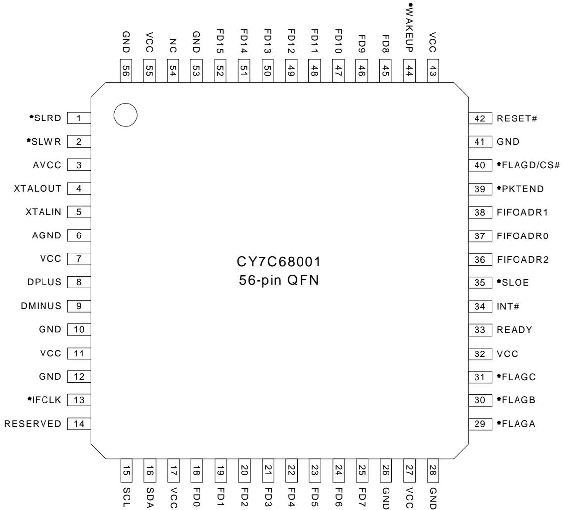
**Figure 6-2. CY7C68001 56-pin QFN Assignment<sup>[7]</sup>**
