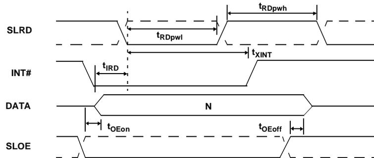
**Figure 11-3. Command Asynchronous Read Timing Diagram<sup>[12]</sup>**
