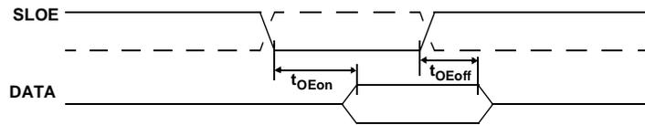
Figure 11-14. Slave FIFO Output Enable Timing Diagram<sup>[11]</sup>
