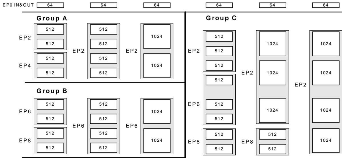
**Figure 3-1. Endpoint Configuration**
