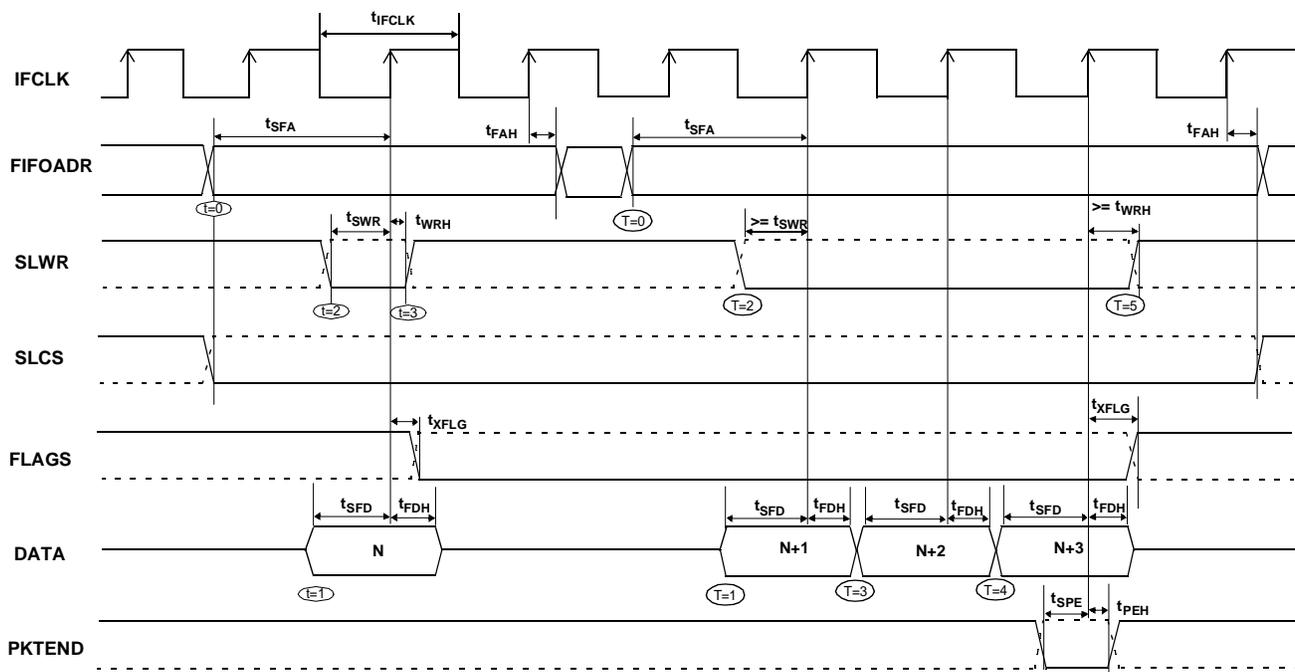
**Figure 11-17. Slave FIFO Synchronous Write Sequence and Timing Diagram<sup>[12]</sup>**
