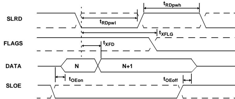
**Figure 11-9. Slave FIFO Asynchronous Read Timing Diagram<sup>[12]</sup>**
