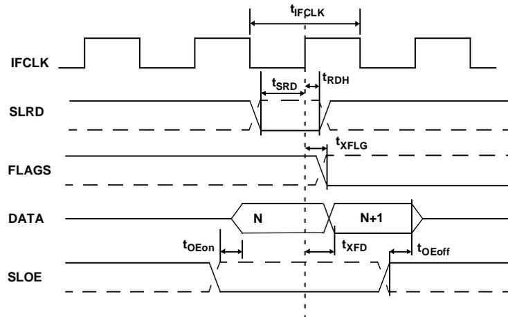
**Figure 11-5. Slave FIFO Synchronous Read Timing Diagram<sup>[12]</sup>**
